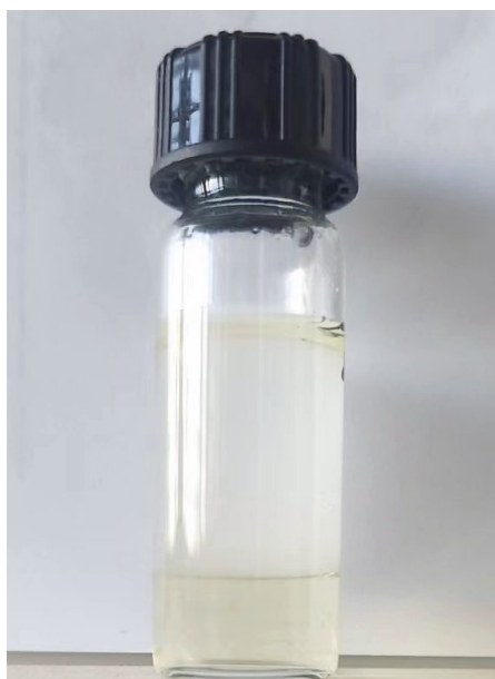
Figure S2. The SIG loaded with sulphur compounds was dissolved in THF and then stratified after adding water.
