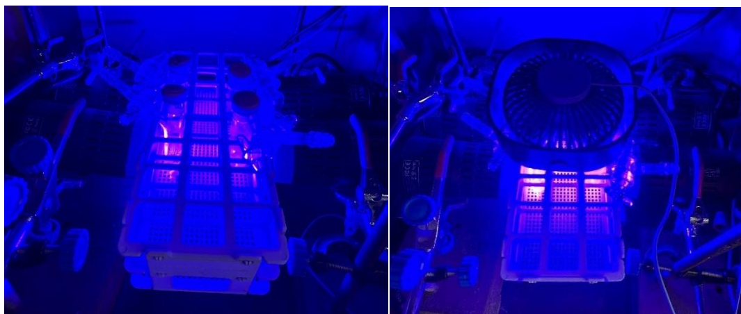
Fig. S1 Kessil reaction setup. reaction was performed under room temperature controlled by fans.
