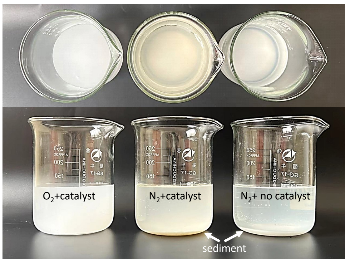
Fig.S8 A comparison of oxidizing MCC products in the presence and/or absence of O 2 as an oxidant. The figures show the front view and top view of the cellulose samples dispersed in deionized water after standing for 1 h, respectively. ( Left :0.5 g MCC, 10 mL DMSO, 4 MPa O 2 , VO(OiPr), 120°C, 12 h ; middle: 0.5 g MCC, 10 mL DMSO, 4 MPa N 2 , VO(OiPr), 120°C, 12 h; right: 0.5 g MCC, 10 mL DMSO, 4 MPa N 2 , 120°C, 12 h. )
