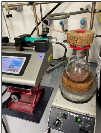
Fig. S25: Reaction setup for the preparative scale reaction on 50 mL scale: \text{H}_2\text{O}_2 was added continuously via a syringe to the reaction mixture in a 250 mL reaction flask. The reaction mixture was stirred using a magnet stirrer.
