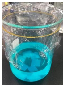
Figure S4. the process of the chitin organogel chelated with Cu 2+ in the Cu(OTf) 2 -containing acetone solution
