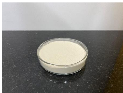
Figure S1. The crab shells after purification are pale yellow chitin powder.
