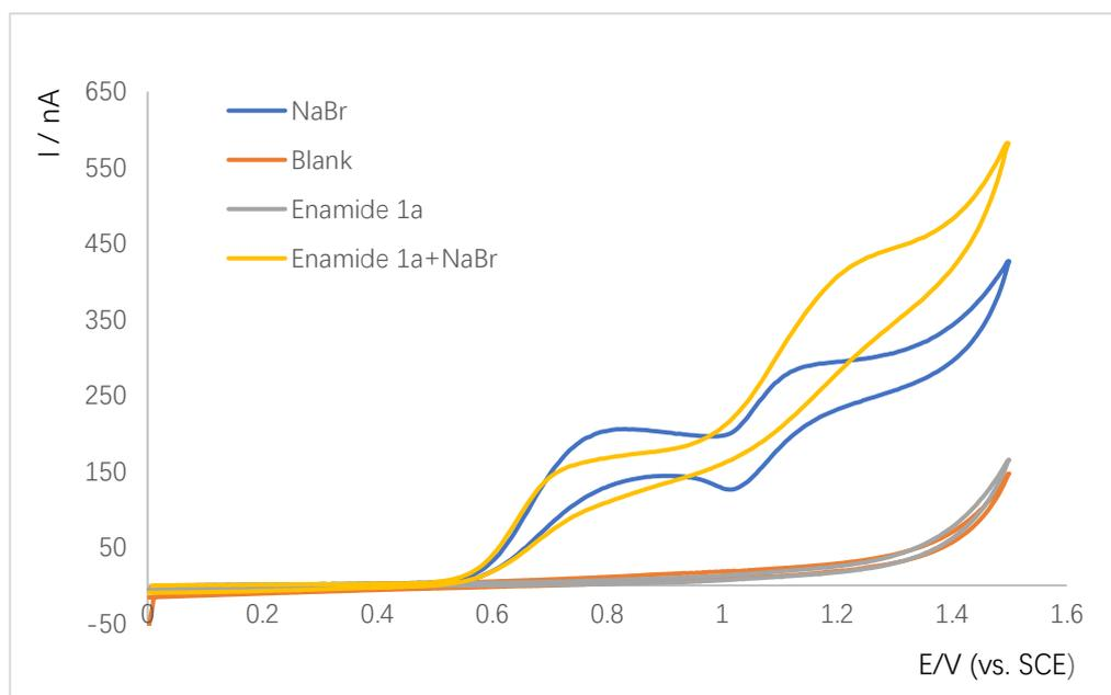
**Figure S2.** CV curve for a solution of 0.01 M NaBr/0.01M Enamide and 0.05 M  $n\text{Bu}_4\text{NBF}_4$  in DMA on a Pt working electrode ( $d = 0.1$  mm), Pt wire ( $d = 1$  mm) auxiliary electrode, SCE reference electrode under a scan rate of 0.1 V/s ranging from 0 V to 1.5 V in oxidation. Following IUPAC CV plotting convention.
