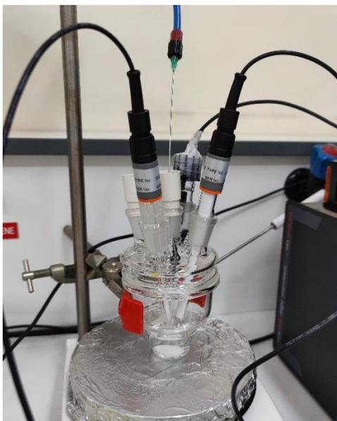
**Figure S1.** Cyclic voltammetry cell.
