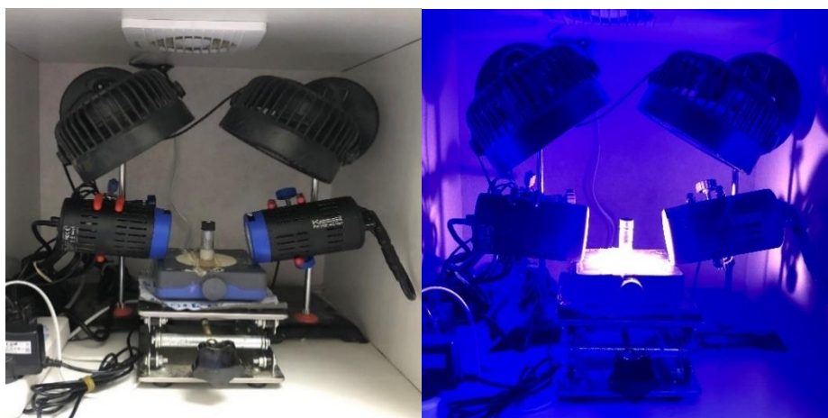
Figure S1. Reaction setup for hydrodefluorination and defluoroallylation of trifluoromethylarenes reaction using 427 nm Kessil Lamp.
