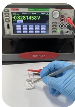
**Figure S10.** The illustrative diagram of self-powered hydrogel batteries still outputs normal voltage when subjected to mechanical damage.
