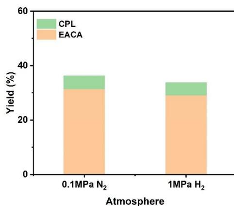
Figure S1. PCL depolymerization with Ru/CeO<sub>2</sub> under different atmosphere. Reaction conditions: PCL, 1 mmol; Ru/CeO<sub>2</sub>, 50 mg; NH<sub>3</sub>·H<sub>2</sub>O, 3 mL; 18h, 140 °C.
