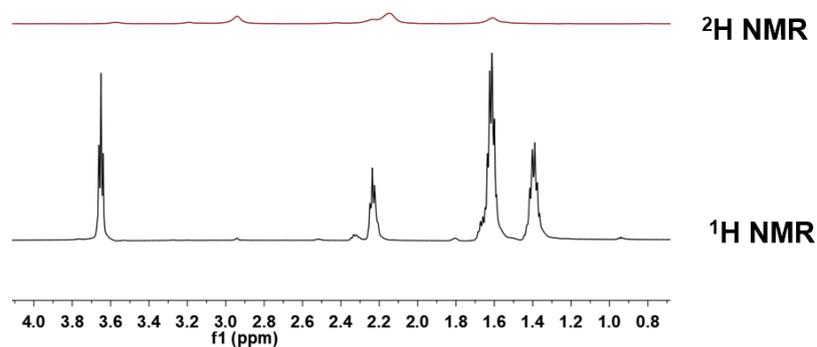
Figure S11. Amination experiment of PCL in ND<sub>3</sub>-D<sub>2</sub>O. Reaction conditions: PCL, 1 mmol; Ru/CeO<sub>2</sub>, 50 mg; ND<sub>3</sub>-D<sub>2</sub>O, 1 mL; 140 °C, 18 h. (<sup>2</sup>H NMR: H<sub>2</sub>O as solvent, <sup>1</sup>H NMR: D<sub>2</sub>O as solvent; room temperature).
