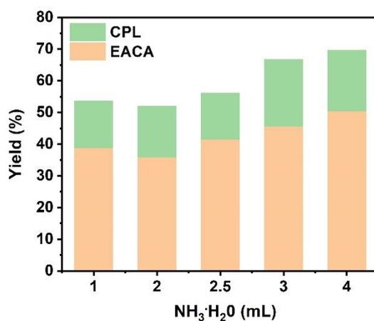
Figure S2. PCL depolymerization using different amount of NH<sub>3</sub>·H<sub>2</sub>O over Ru/CeO<sub>2</sub>. Reaction conditions: PCL, 1 mmol; Ru/CeO<sub>2</sub>, 50 mg; 18h, 160 °C.
