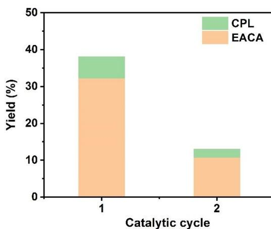
**Figure S6. Recycling experiment of Ru/CeO<sub>2</sub> as a catalyst for PCL degradation.** Reaction conditions: PCL, 1 mmol; Ru/CeO<sub>2</sub>, 50 mg; NH<sub>3</sub>·H<sub>2</sub>O, 3 mL; 140 °C, 18 h for each cycle. Note: The catalyst was separated from the reaction system by centrifugation and washed with water and ethanol for 3 times. After being dried under vacuum, the recovered catalyst was reused for the next run.
