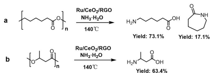
**Figure S7. (a) PCL degradation.** Reaction conditions: PCL, 0.2 mmol; Ru/CeO<sub>2</sub>/RGO, 10 mg; NH<sub>3</sub>·H<sub>2</sub>O, 1 mL; 140 °C, 144 h. **(b) PHB degradation.** Reaction conditions: PHB, 0.2 mmol; Ru/CeO<sub>2</sub>/RGO, 10 mg; NH<sub>3</sub>·H<sub>2</sub>O, 1 mL; 140 °C, 18 h.
