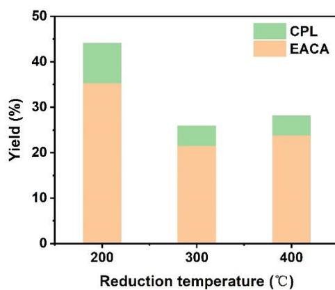
**Figure S4.** PCL depolymerization over Ru/CeO<sub>2</sub> reduced at different temperatures. Reaction conditions: PCL, 1 mmol; Ru/CeO<sub>2</sub>, 50 mg; NH<sub>3</sub>·H<sub>2</sub>O, 3 mL; 18 h, 140 °C.
