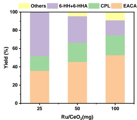
**Figure S3.** PCL depolymerization over Ru/CeO<sub>2</sub> using different catalyst dosage. Reaction conditions: PCL, 1 mmol; NH<sub>3</sub>·H<sub>2</sub>O, 3 mL; 18 h, 160 °C.
