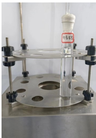
Fig. S12 Schematic diagram of hydrogen evolution device.
