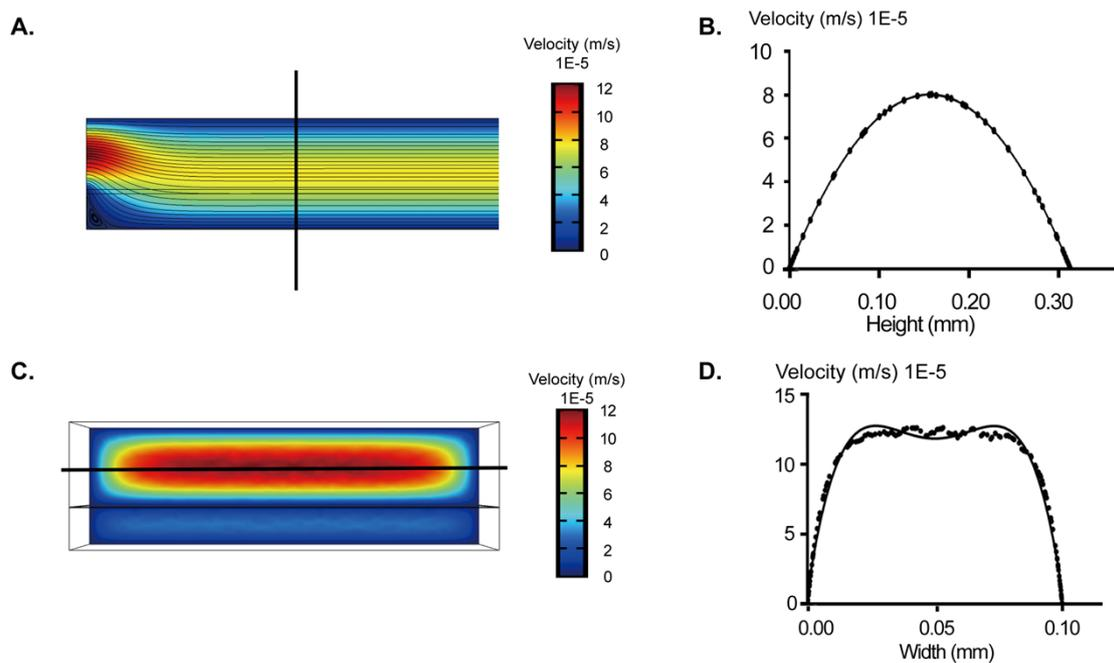
**Figure S1.** Computational flow filed in the hBCSFB-on-chip in the absence of cells in different profiles. (A) Velocity profile at the section Z-X in  $X=0.5$  mm (the second half of the section was omitted). (B) Computational velocity profile at the section Z-X. (C) Velocity profile at the section Z-Y in  $X=0.1$  mm. (D) Computational velocity profile at the section Z-Y.
