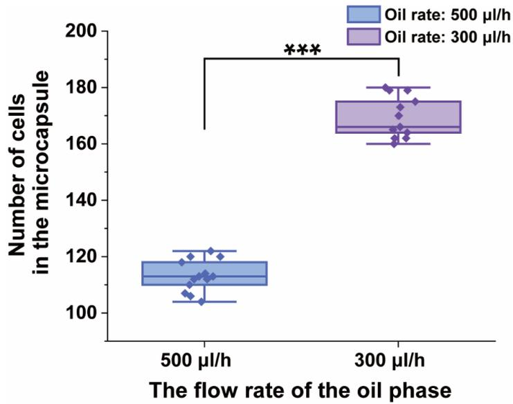
**Fig. S7.** Quantification of initial cell loading of different sizes of cell-laden microcapsules. The cell-laden microcapsules were generated at the flow rate of the oil phase fixed at 300  $\mu\text{l h}^{-1}$  and 500  $\mu\text{l h}^{-1}$  respectively. (N=13, \*\*\*P < 0.001).
