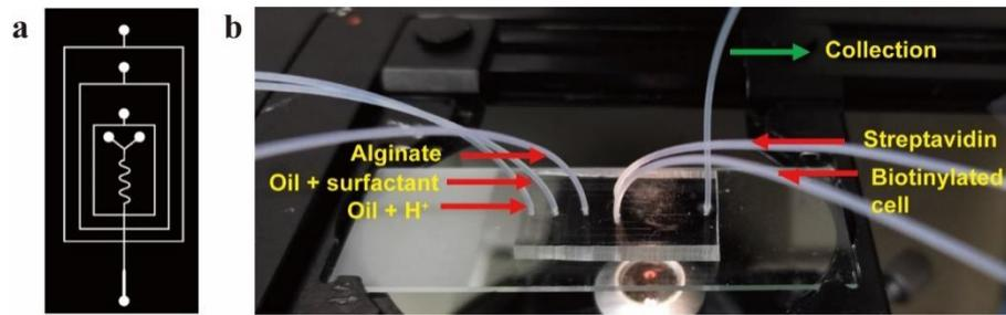
**Fig. S1.** Design and operation of the microfluidics device. (a) The mask design of the microfluidics device. (b) Device diagram for microcapsules generation.
