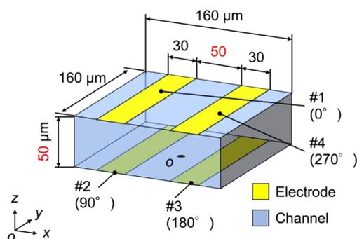
Fig. S1 Schematic of calculation domain for electric field simulation.
