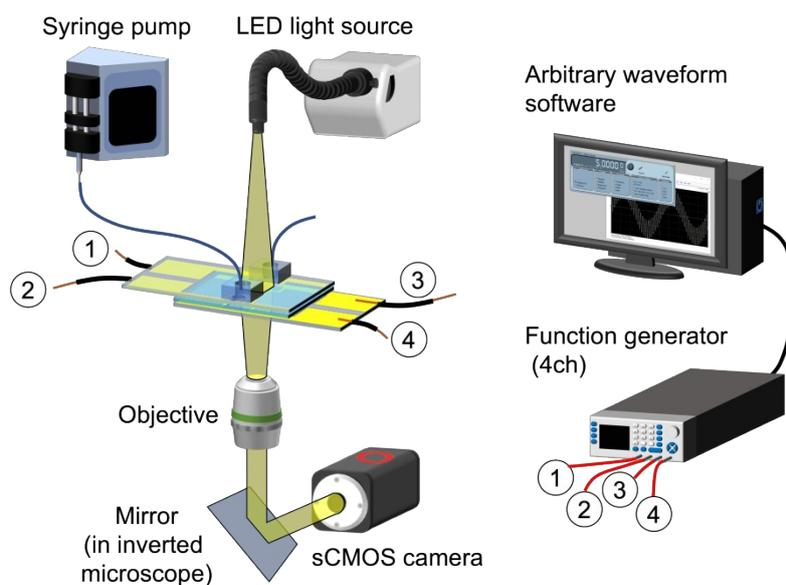
Fig. S1 Schematic of setup for cROT experiment.
