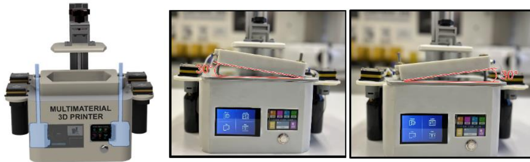
Figure SI2 - Position of the two stepper motors and vat inclination system.
