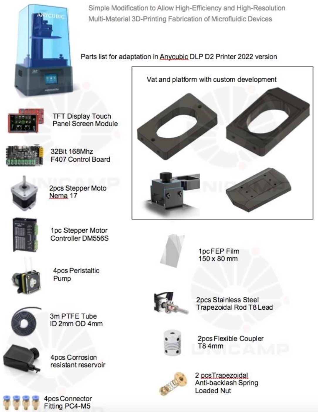
Figure SI9 – Parts list for adaptation of Anycubic DLP D2 printer 2022 version.
