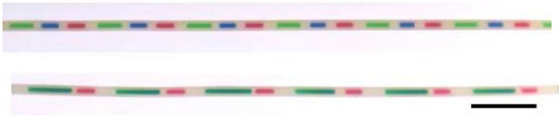
**Fig. S5 (Caption)** Video of the mergings of droplets. Top shows the first merging, bottom the second. Droplets were made of food coloring diluted in water. A fast flow ( $5\mu\text{L/s}$ ) is applied, then a slow flow ( $0.3\mu\text{L/s}$ ) to bring the droplets back to their initial position. This operation is repeated twice for each merging. Speed  $\times 10$ . Scale bar: 1cm.
