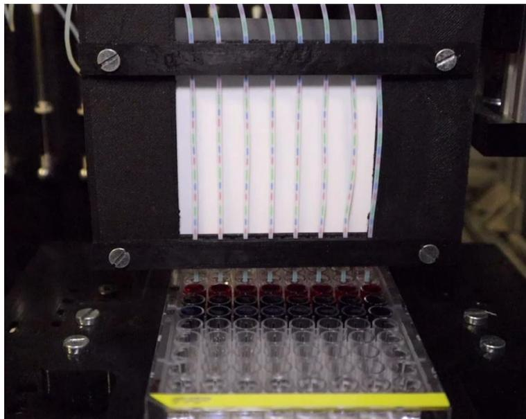
**Fig. S3 (Caption)** Video of the drug screening platform during filling of 8 tubes with colored droplets (food coloring in water). Real speed.
