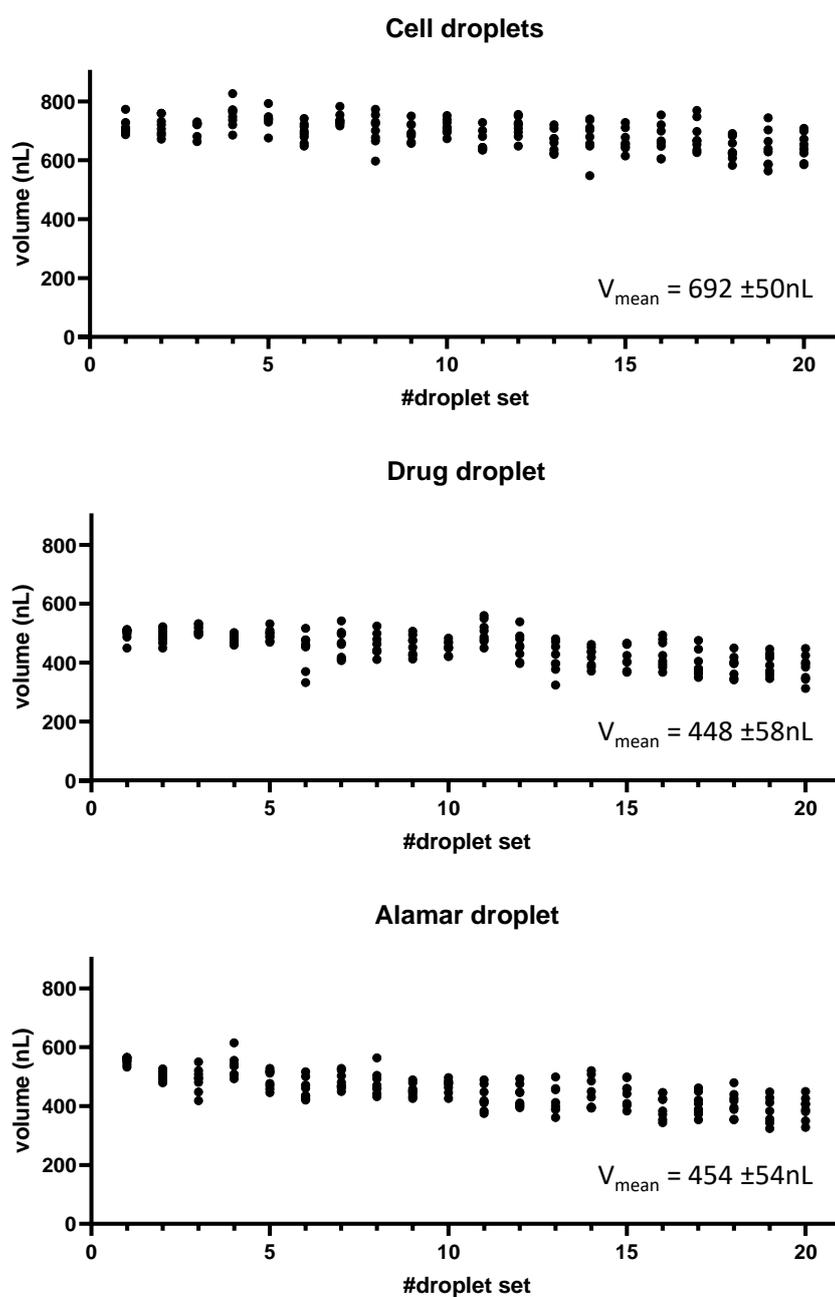
**Fig. S4** Volumes of cell, drug and alamar droplets. Droplets were generated by pipetting 20 trains of colored droplets in each of the 8 tubes in parallel. Volumes were computed from the length of the droplets measured on fluorescence images of the tubes.
