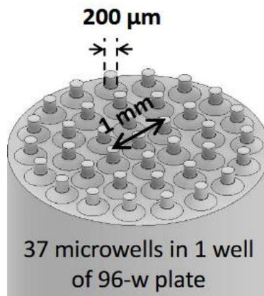
**Fig. S2** Scheme of the stamp for agarose microwells production. 34 pillars of diameter 200 $\mu\text{m}$  are distributed over a cylinder fitting in a well of a 96-wells plate.
