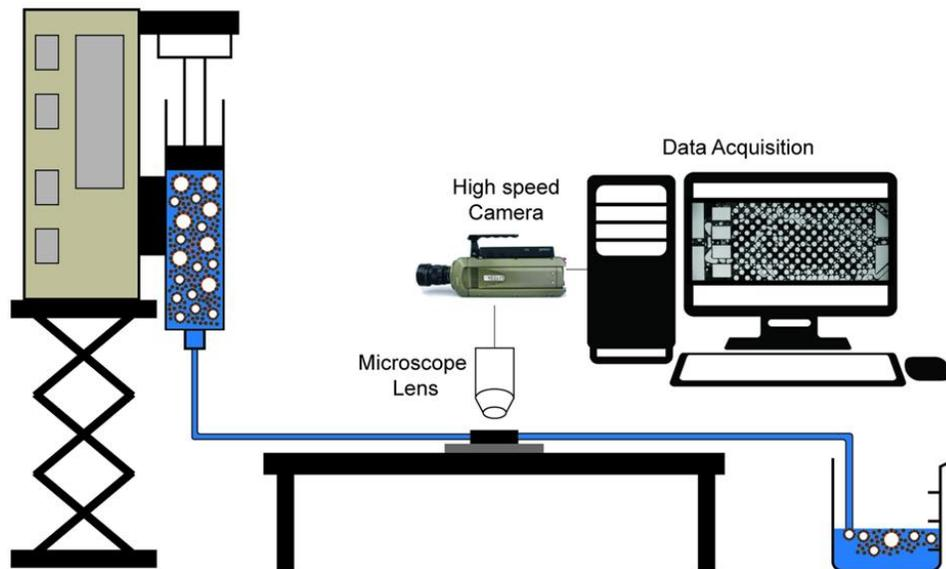
Fig. S1: Apparatus and set-up used to image capillary foam flow.
