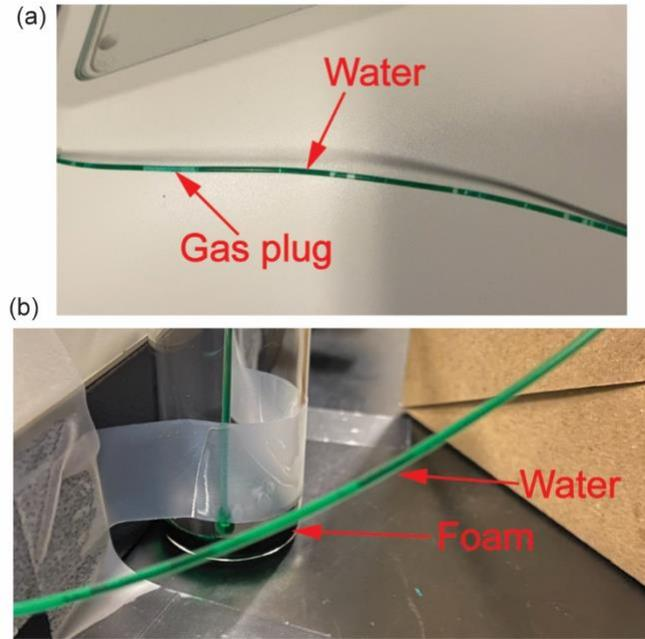
Fig. S2: Images of capillary foams dyed with green food dye flowing through a polyethylene tube showing phase separation between (a) water and gas, (b) foam and water before entering the micromodel.
