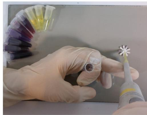
Injection of amino acid solution in the central zone and then scanning the PAD
