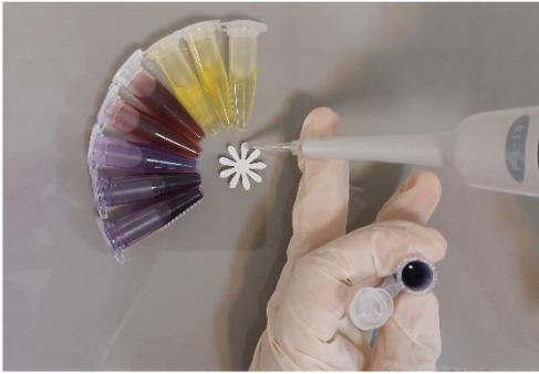
Injection of the sensing elements on the paper petals
