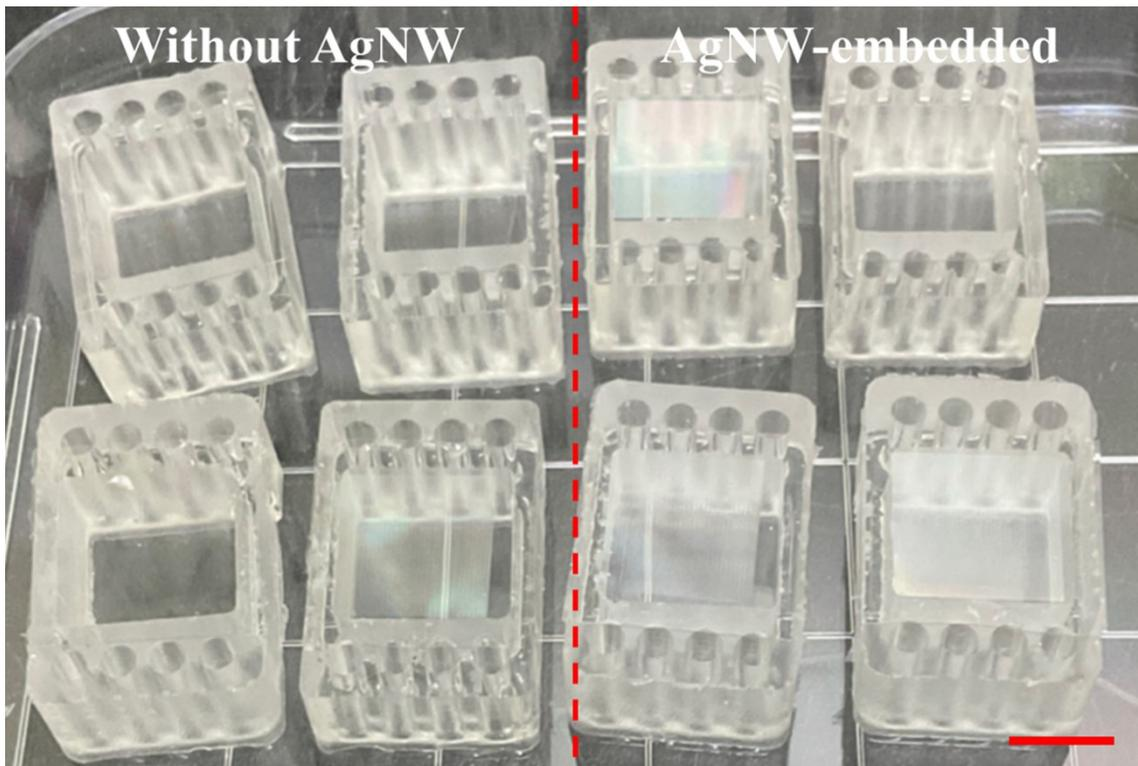
Fig. S4. Photograph shows the fabricated PDMS functional well plate, presented in two variations: one without and another with AgNWs embedded within the microgrooved PDMS membrane (Scale bar: 1 mm).
