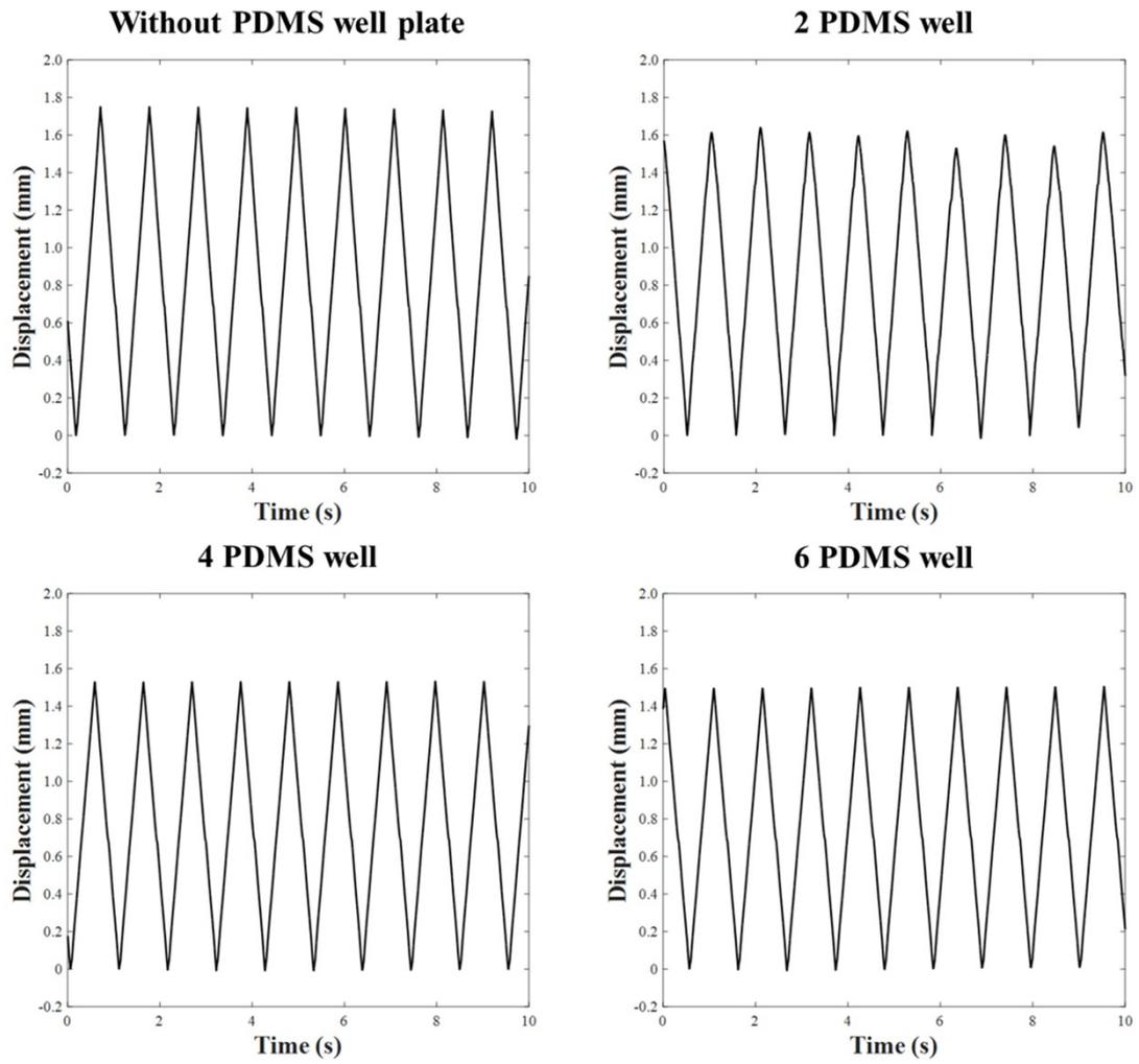
Fig. S8. Real-time traces illustrating the displacement variations of the moving plate, corresponding to the number of PDMS well plates, under a 10% applied tensile stress with 1 Hz mechanical stimulation.
