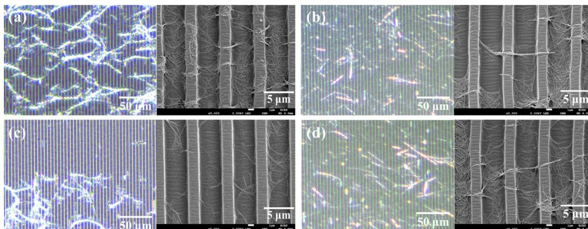
Fig. S6. Optical and FE-SEM analysis of the AgNWs-S-PDMS and AgNWs-E-PDMS membrane before (a, b) and after (c, d) peeling test using 3 M adhesive tape.
