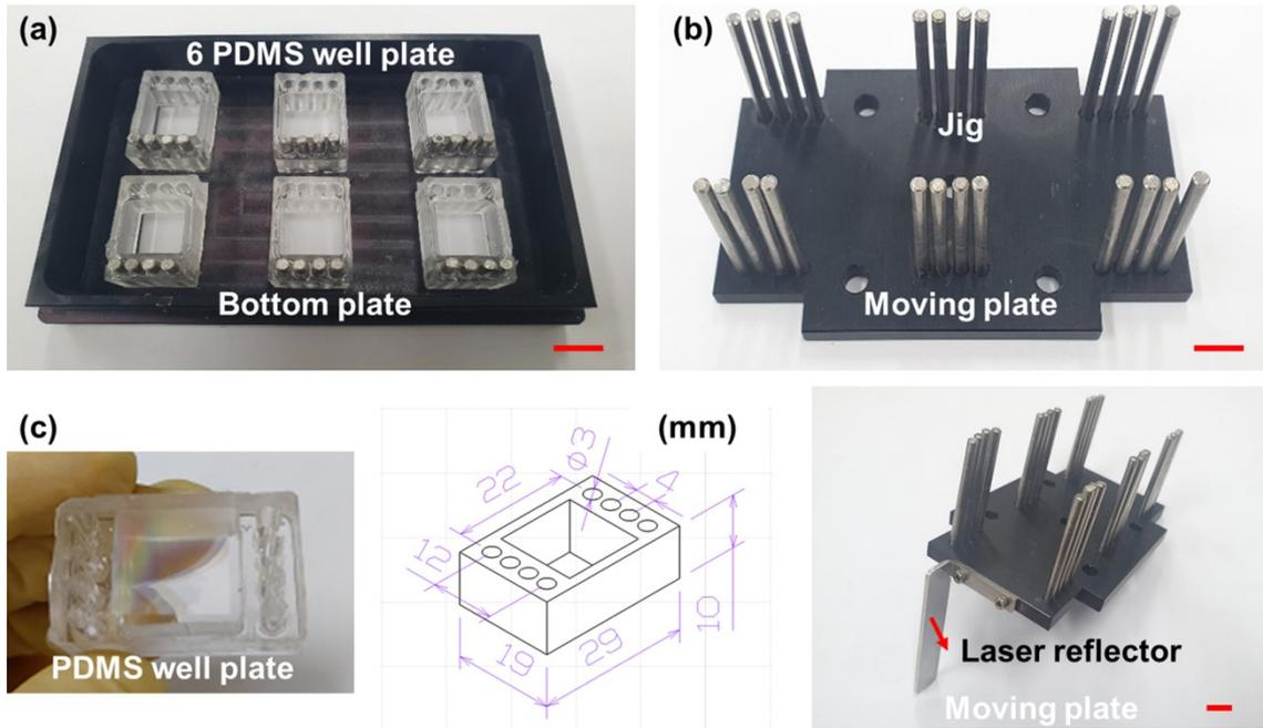
Fig. S2. Photographs show the various parts of the mechanical stimulation system such as (a) PDMS well plate, (b) moving plate, (c) PDMS well plate and laser reflecting sensor in the moving plate. (Scale bar: 1 mm)
