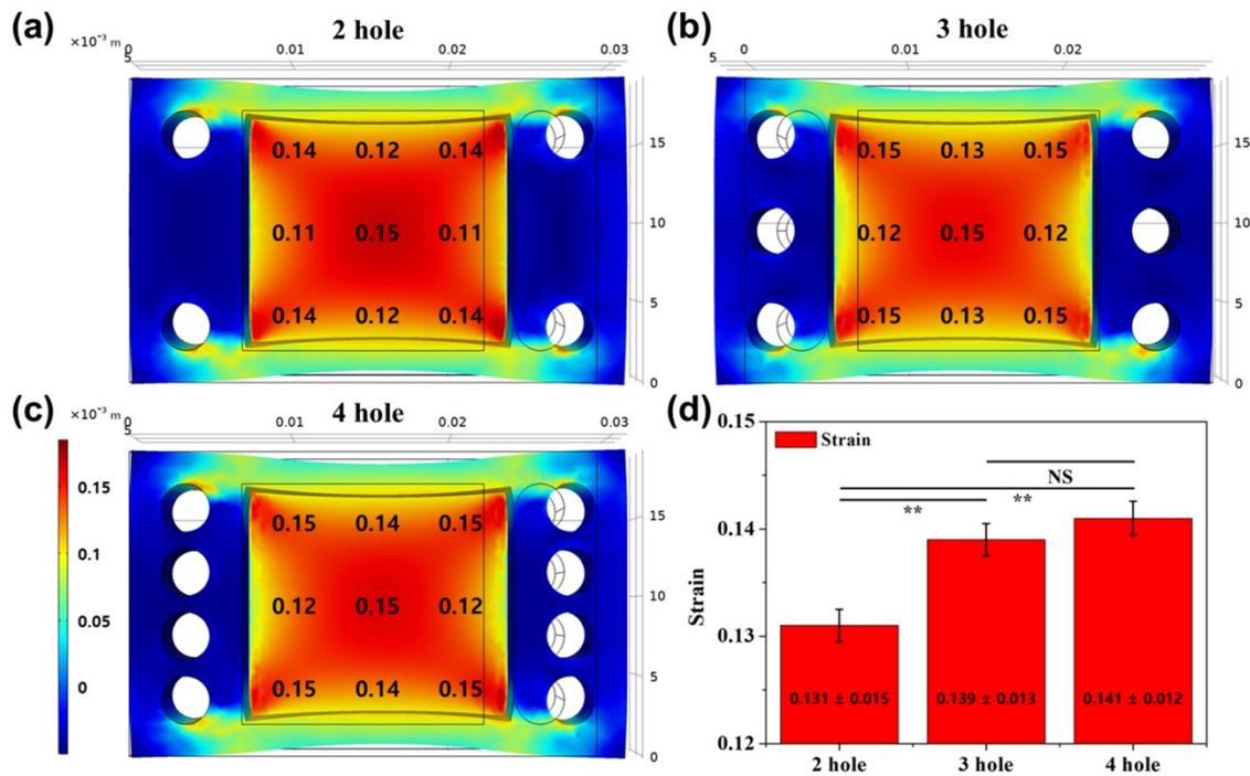
Fig. S3. (a-c) Finite Element Method (FEM) simulation analysis of the proposed PDMS membrane with 15 mm in length x 15 mm in width x 100 μm in thickness, employed to evaluate stress distribution across the membrane. (d) Bar plot depicting strain distribution on the PDMS membrane according to number of jigs. Data represented as mean ± standard deviation (n = 6). The bars and error bars indicate the mean ± standard deviation (n = 6). \*P < 0.05, \*\*P < 0.01.
