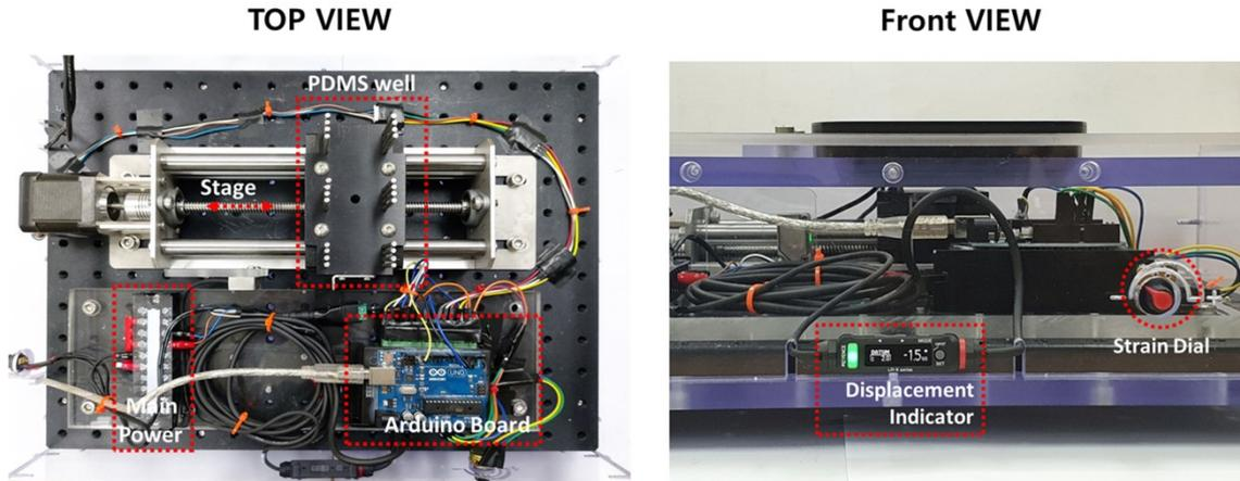
Fig. S1. Photographs show the top and front view of the proposed mechanical stimulation system.
