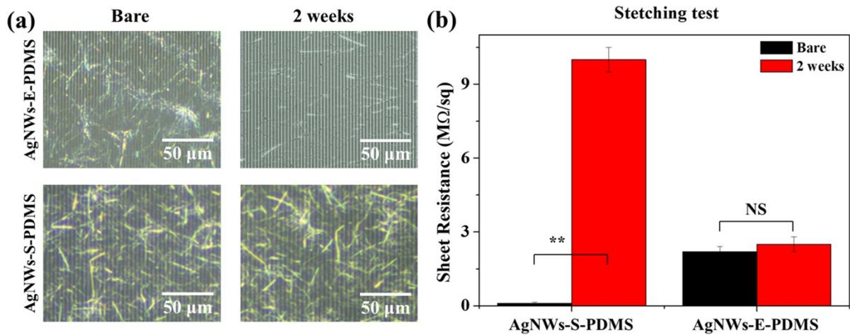
Fig. S7. Structural integrity and sheet resistance of the AgNWs-S-PDMS and AgNWs-E-PDMS membranes before and after sustained cyclic mechanical stretching at 1 Hz for 2 weeks. The bars and error bars indicate the mean  $\pm$  standard deviation ( $n = 6$ ). NS (Non-significant),  $*P < 0.05$ ,  $**P < 0.01$ .
