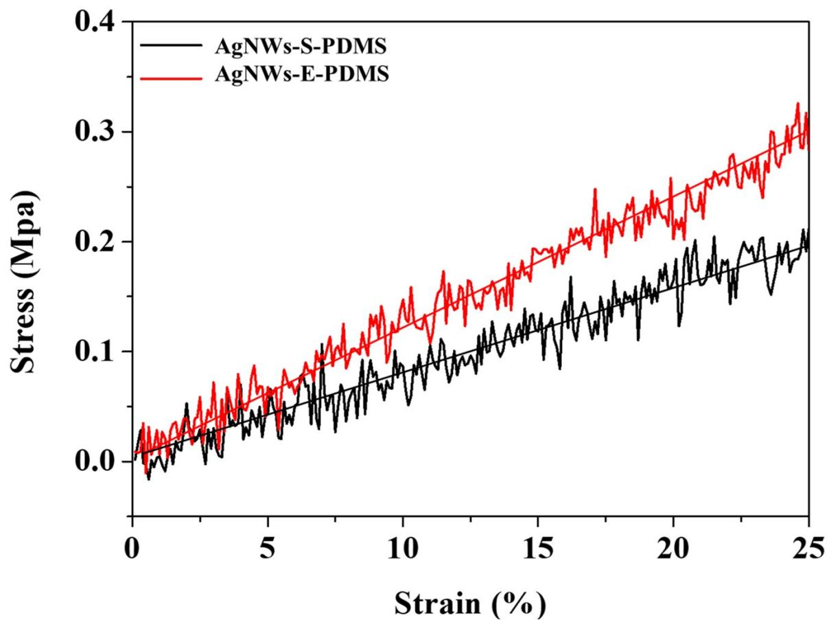
Fig. S9. Stress-strain profile demonstrate the tensile strength of the AgNWs-S-PDMS and AgNWs-E-PDMS membranes.
