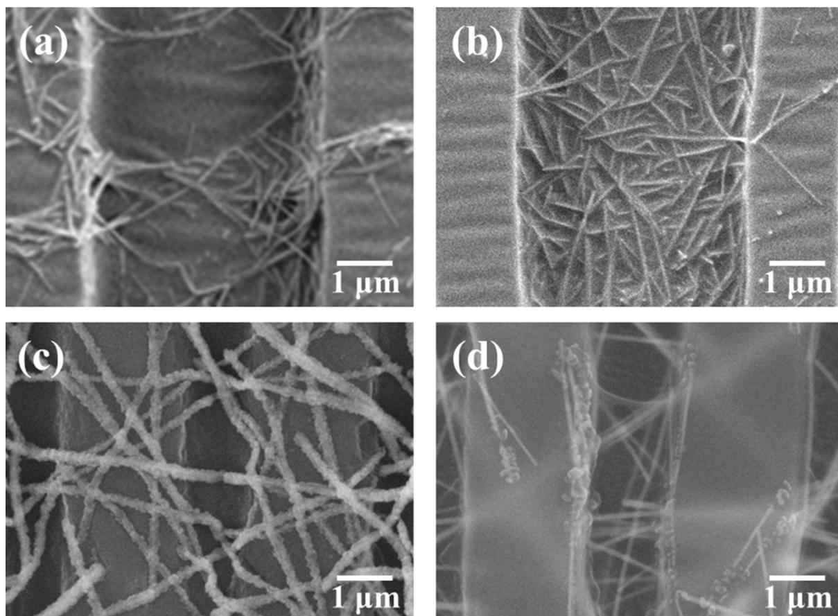
Fig. S5. FE-SEM analysis of the AgNWs-S-PDMS and AgNWs-E-PDMS membrane before (a, b) and after (c, d) exposed to oxygen plasma treatment at 100 W for 1 min.
