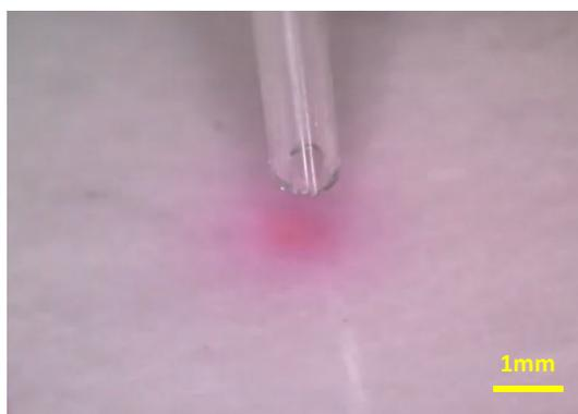
**Figure S2.** Enrichment of rhodamine in ethanol after 2 minutes. 20  $\mu\text{L}$  of rhodamine solution was deposited on a hydrophilic glass surface, and 1  $\mu\text{L}$  of a 1% PDMS solution in hexane was added to the surface of the solution.
