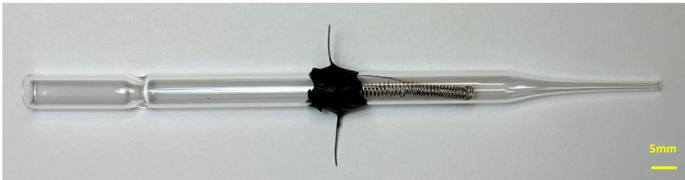
**Figure S3.** Image of the heated airjet nozzle used for enrichment. The nozzle consists of two halves of a borosilicate glass pipette with the heating element inserted in the middle. The heating element consists of a 40 mm coil nichrome that is braided at the ends with wire. The glass halves are then sealed with ceramic adhesive.
