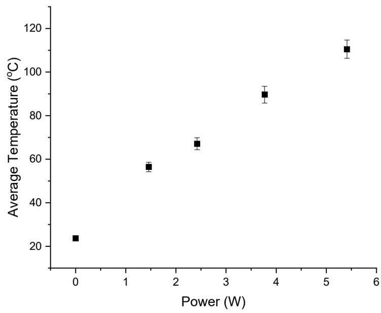
**Figure S4.** Average temperature vs. power for the pipette's exit nozzle
