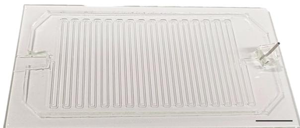
**Figure S1.** A representative photograph of the modified droplet collection chip. Scale bar: 20 mm.
