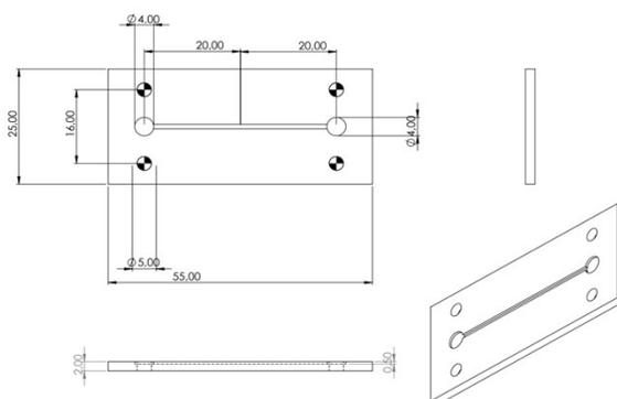
Fig. S2 True to scale drawing of the bottom part of the chip.
