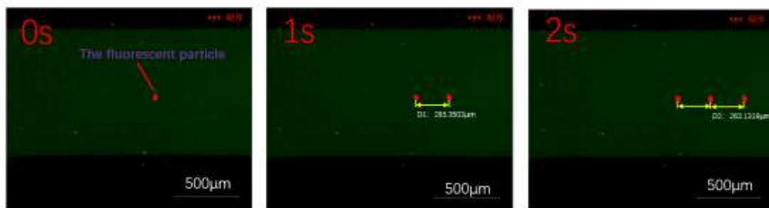
Fig. S8. The fluid velocity measurement method on the chip based on the fluorescent microparticle. The motion video of the polystyrene particles was acquired under a fluorescence microscope, and the video editing software was used to obtain the picture of each frame. And then the Image-pro-plus software was used to measure the moving distance of each fluorescent particle at each time interval to obtain the particle motion speed. Multiple fluorescent particles in the microchannel were selected to calculate the average velocity of the fluid. Scale bar: 500 \mu\text{m} .
