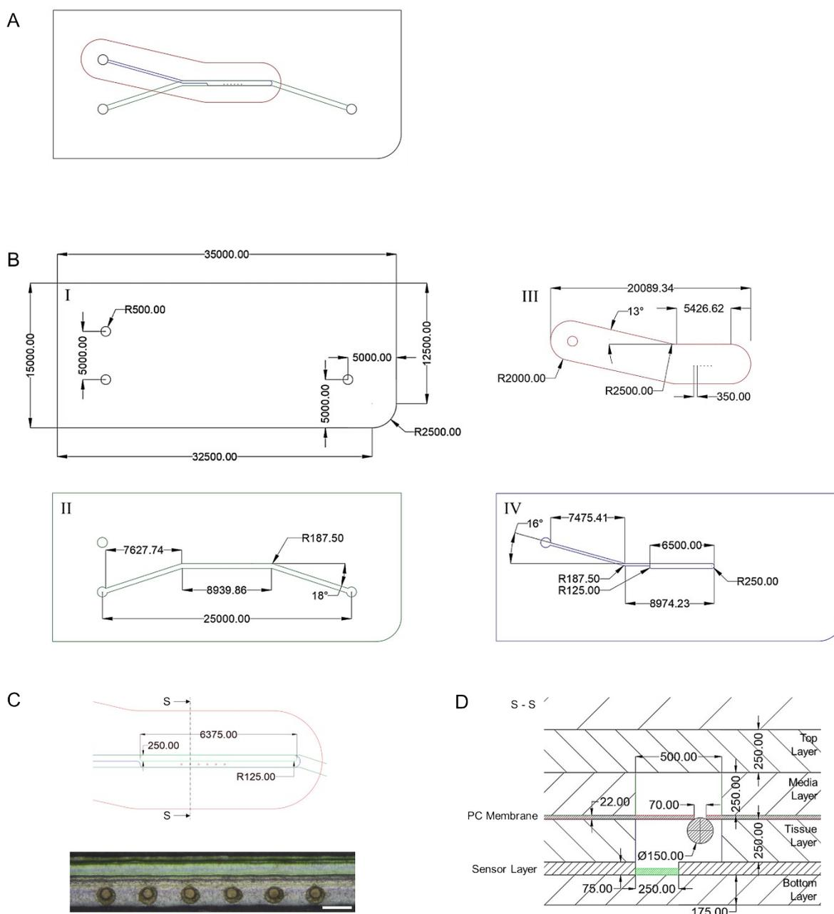
Figure S1: Microfluidic chip set-up and design. (A) Top view of all chip layer drawings showing the alignment of tissue and media channel. (B) Dimensioned drawings of all chip layers (in  $\mu\text{m}$ ; top layer (I), media layer (II), membrane (III) and tissue layer (IV)). The PDMS connection layer has the same dimensions
