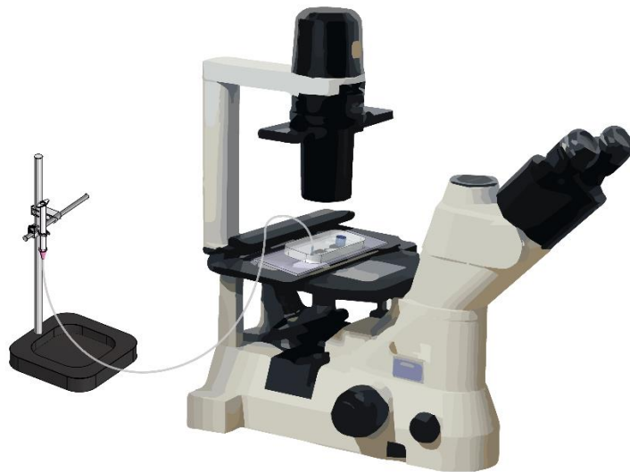
Fig. S1 The experimental setup included the microscope, the microfluidic device, and the syringe containing mHTF buffered medium. The height of the syringe is adjusted with respect to the device surface to control the flow rate.
