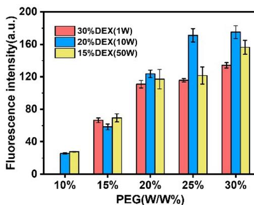
**Figure S4.** The fluorescence intensity map of DEX and PEG enriched miRNA with varying mass fraction and molecular weight. The fluorescence intensity of 30% DEX (10000), 20% DEX (100000), and 15% DEX (500000) was measured after enrichment through mixing with 10%, 15%, 20%, 25%, and 30% PEG (8000). Volume ratios=1:15, pH=9.0.
