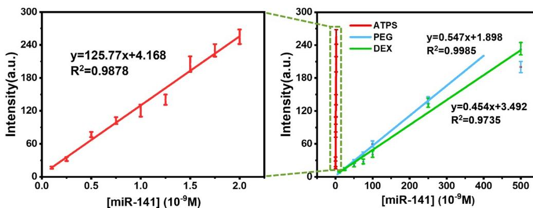
**Figure S10.** A linear correlation between the intensity of the red fluorescence signal and the concentration of miRNA-141 in ATPS microdroplet and, single-phase PEG and DEX systems.
