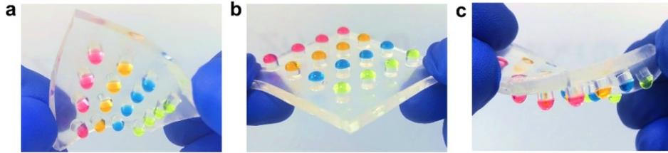
**Figure S1.** Performance of the PDMS minipillar array. Whether (a) bent, (b) stretched, or (c) twisted, the droplets can be securely anchored to the minipillar array.
