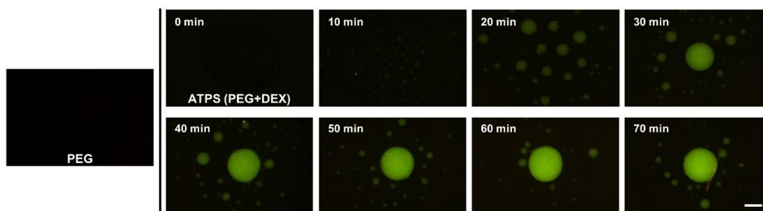
**Figure S5.** The volume of the DEX-rich phase increased gradually during the static phase separation, and the fluorescence intensity also increased gradually. Scale bar: 500  $\mu\text{m}$ .
