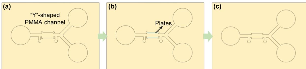
**Fig. S7** (a) The manufacturing drawing of the “Y”-shaped PMMA channel; (b) The “Y”-shaped PMMA channel with two plates; (c) The final shape of the “Y”-shaped PMMA channel channel.
