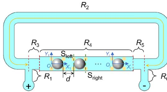
**Fig. S5** Schematic diagram of a multi-droplet cuboid pump.  $d$  is the distance between two adjacent droplets. Changes in the number of droplets affect the shape of the solution in the corresponding area of  $R_4$ .
