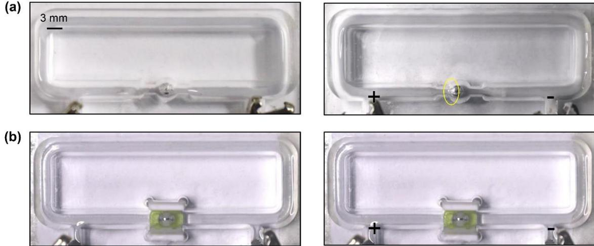
**Fig. S3** (a) The morphologies of the droplet in the cylindrical pump without (left) and with (right) an electric field. (b) The morphologies of the droplet in the cuboid pump without (left) and with (right) an electric field.  $V_{p-p}$  is 10 V,  $V_{DC}$  is 5 V,  $f$  is 50 Hz, and  $C$  is 0.4 M.
