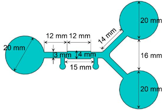
**Fig. S8** Dimensions of the “Y”-shaped PMMA channel
