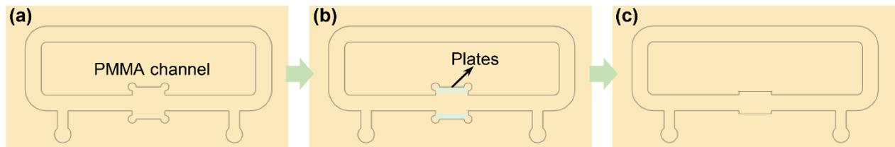
**Fig. S1** (a) The manufacturing drawing of the PMMA channel; (b) The PMMA channel with two plates; (c) The final shape of the PMMA channel.
