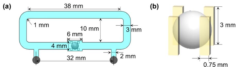
**Fig. S2** (a) Structure and dimensions of the single-droplet cuboid pump, and the height of the microfluidic channel is 6 mm; (b) Dimensions of the pillars.
