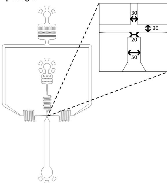
Figure S1. Microfluidic flow focusing design with dimensions depicted in  $\mu\text{m}$ .
