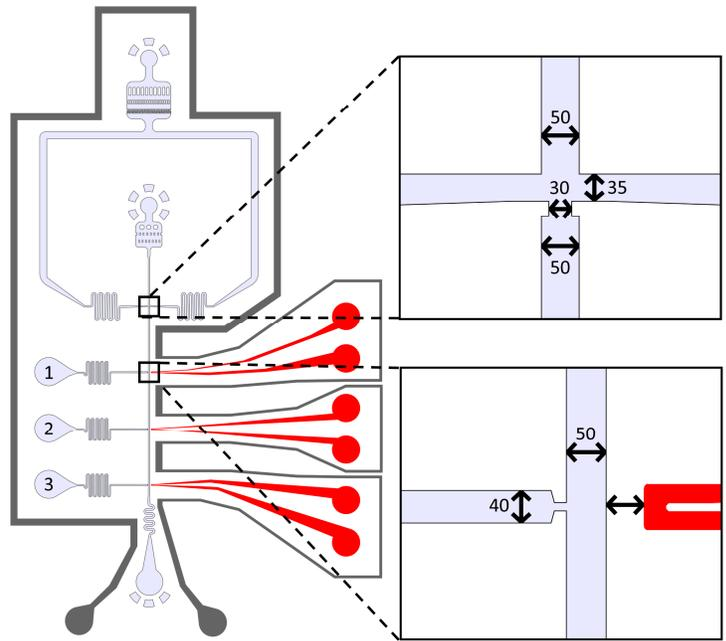
Figure S2. Picoinjection design with the most important dimensions in  $\mu\text{m}$ .
