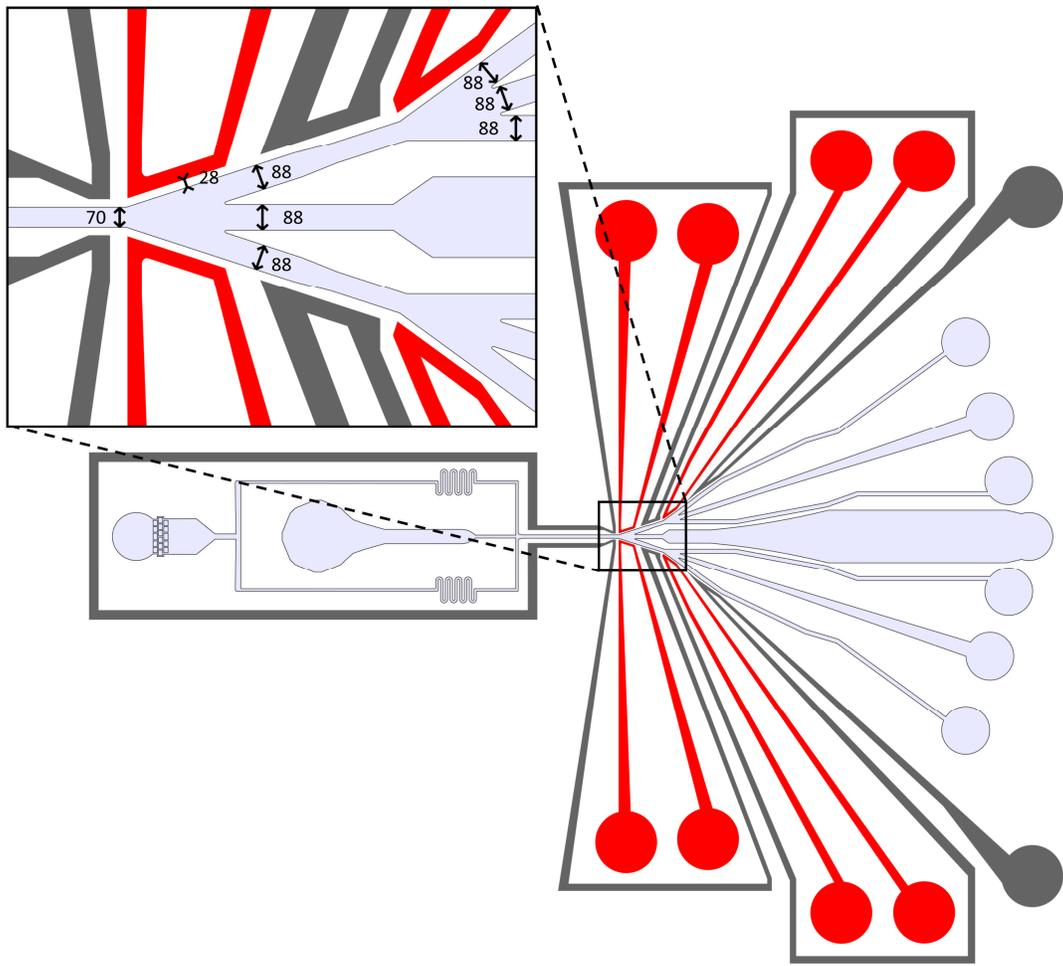
Figure S3. Microfluidic sorting design with the most important dimensions indicated in  $\mu\text{m}$ .
