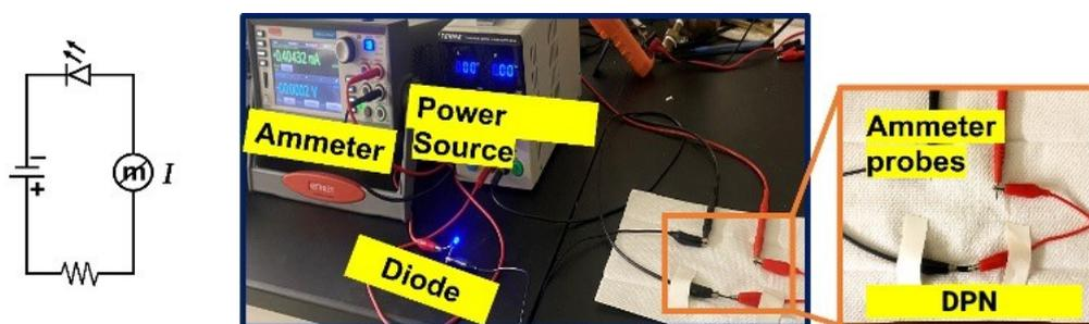
**Figure S6.** Electrical circuit and set-up for measuring current flowing through the circuit using IPN-Lin<sub>100</sub>UPy<sub>7.5</sub>FMA<sub>7.5</sub>2.5%CNT as DPN
