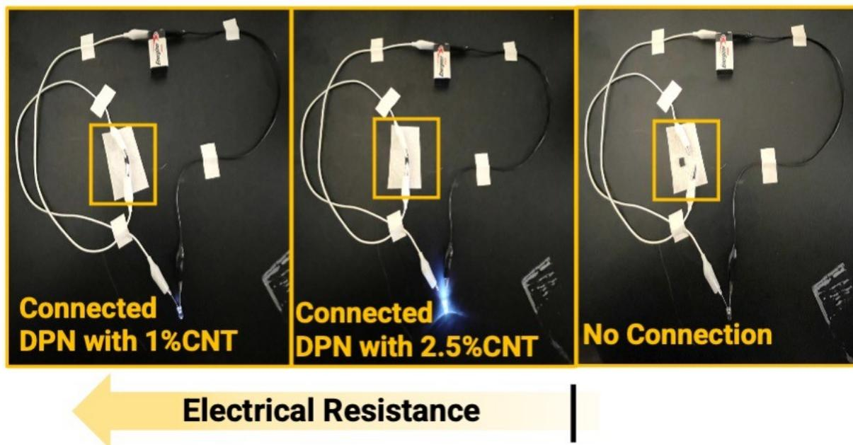
**Figure S7.** Impact of CNT loading on the electrical resistance of IPN-Lin<sub>100</sub>UPy<sub>7.5</sub>FMA<sub>7.5</sub> as DPN in a circuit system.
