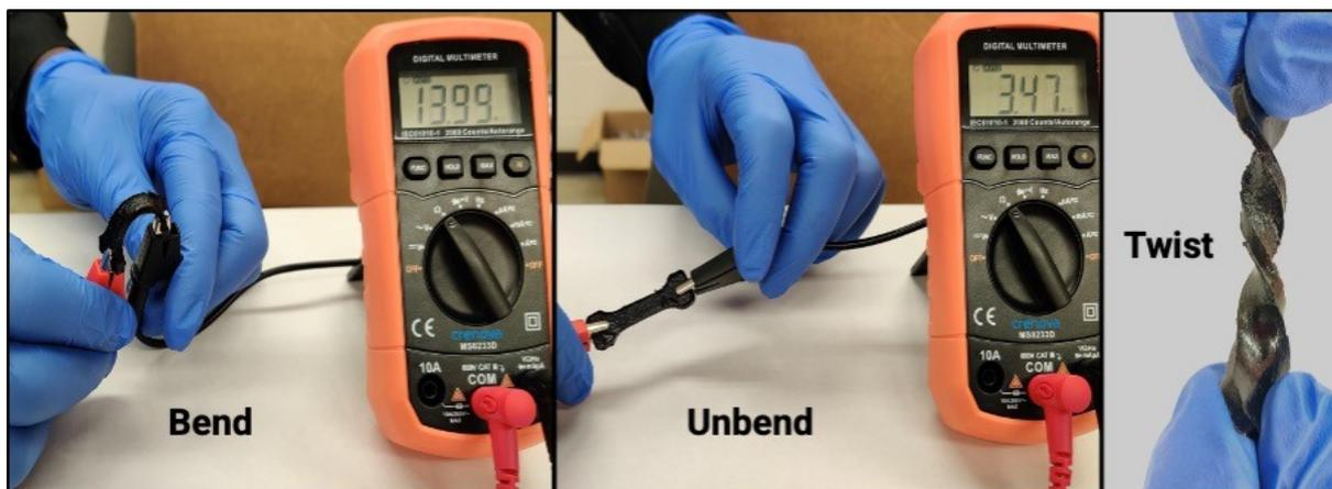
**Figure S10.** IPN-Lin<sub>100</sub>UPy<sub>7.5</sub>FMA<sub>7.5</sub>2.5%CNT attached to a multimeter with bending and unbending photographs. Also twisted IPN-Lin<sub>100</sub>UPy<sub>7.5</sub>FMA<sub>7.5</sub>2.5%CNT is shown with good flexibility.
