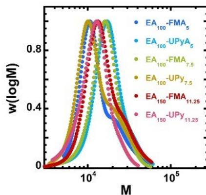
**Figure S1.** GPC traces of IPN precursors: poly(EA<sub>100</sub>-FMA<sub>5</sub>), poly(EA<sub>100</sub>-UPy<sub>5</sub>), poly(EA<sub>100</sub>-FMA<sub>7.5</sub>), poly(EA<sub>100</sub>-UPy<sub>7.5</sub>), poly(EA<sub>150</sub>-FMA<sub>11.25</sub>), and poly(EA<sub>150</sub>-UPy<sub>11.25</sub>). Dispersity data is provided in Table S1.
