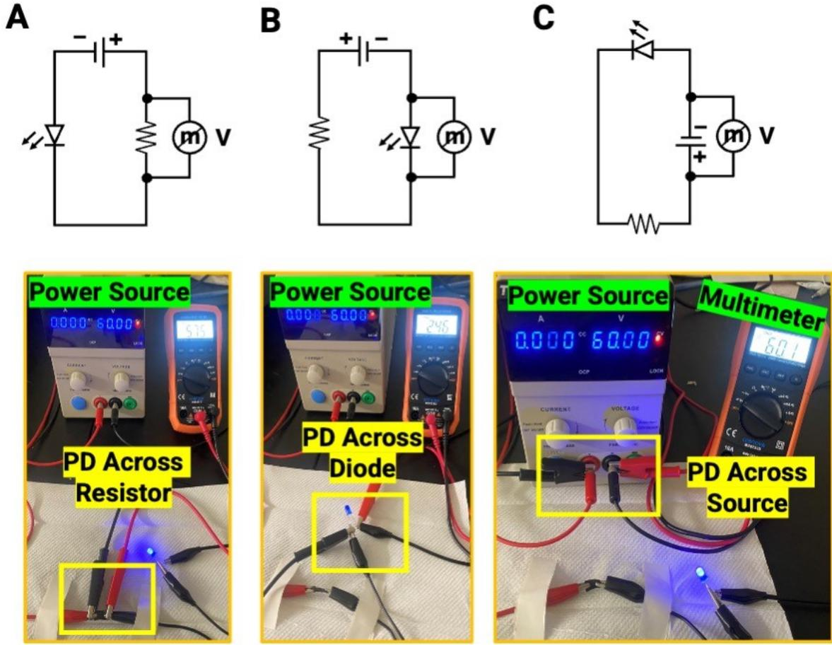
**Figure S9.** Electrical circuits and set-ups showing measurements of PD across (A) resistor, (B) diode, and (C) source.
