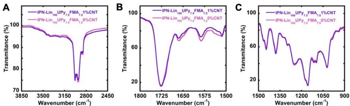
**Figure S4.** Closer look (zoomed-in) IR spectrum for reinforced and unreinforced IPN-Lin<sub>100</sub>UPy<sub>7.5</sub>FMA<sub>7.5</sub> materials.
