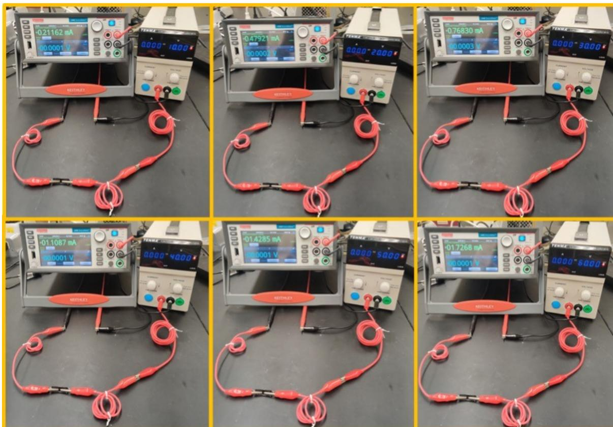
**Figure S11.** Typical set-up for measuring the impact of current on custom resistors using 30%L-70%H with applied voltage of 10, 20, 30, 40, 50, 60 V to obtain current-voltage plot.
