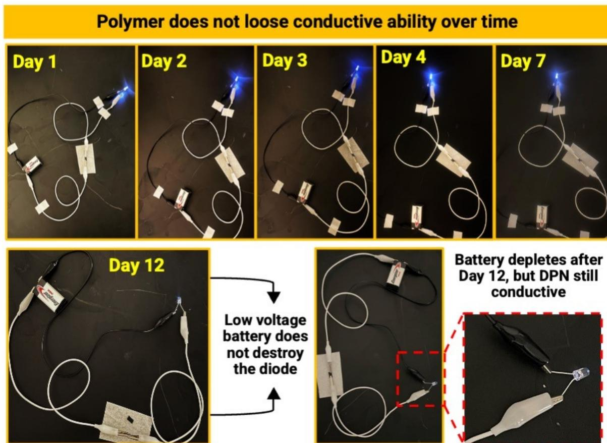
**Figure S8.** Conduction of current through IPN-Lin<sub>100</sub>UPy<sub>7.5</sub>FMA<sub>7.5</sub>2.5%CNT in a circuit system which lasted until circuit battery was depleted.
