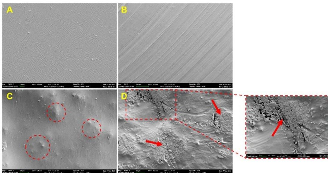
**Figure S5.** Scanning electron micrographs of (A) surface and (B) razor-sliced cross-section of IPN-Lin<sub>100</sub>UPy<sub>7.5</sub>FMA<sub>7.5</sub>0%CNT. (C) Surface and (D) razor-sliced cross-section of IPN-Lin<sub>100</sub>UPy<sub>7.5</sub>FMA<sub>7.5</sub>2.5%CNT.
