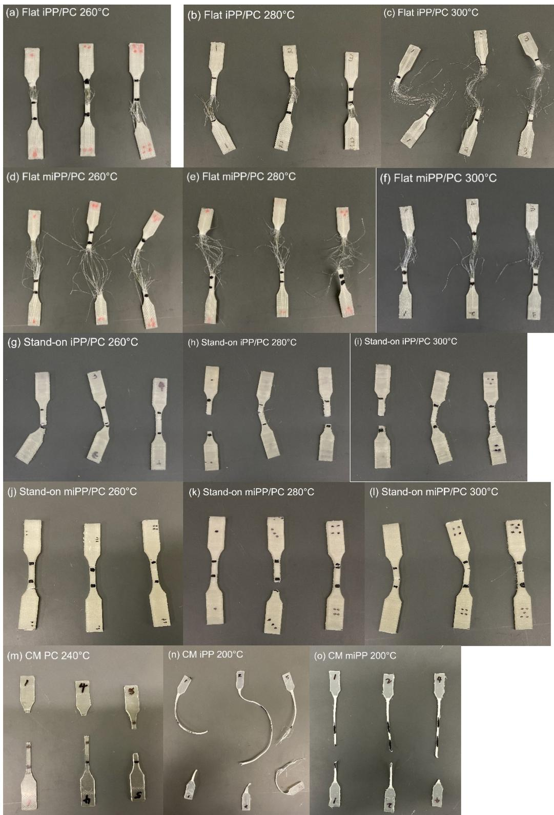
**Figure S12.** Images of the tensile bars post failure for 3D printed in flat orientation iPP (shell)-PC (core) at (a) 260 °C, (b) 280 °C and (c) 300 °C as well as mPP (shell) – PC (core) at (d) 260 °C, (e) 280 °C and (f) 300 °C. Images of the 3D printed tensile bars in stand-on orientation for iPP
