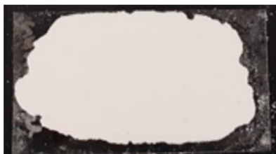
Figure S4. (A) Representative specimen of the ground PMMA-MetCNFs (50:1:0.06) that was compressed on a glass slide at 500 psi for 5 minutes under ambient temperature for static water contact angle measurement. (B) Representative static water contact angle droplet on PMMA-MetCNFs (50:1:0.06) surface at 15 seconds.
