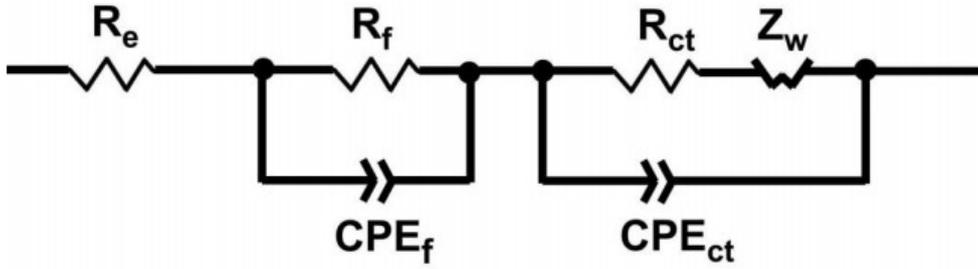
**Figure S5** Equivalent circuit model for Nyquist plots in Figure 4e.
