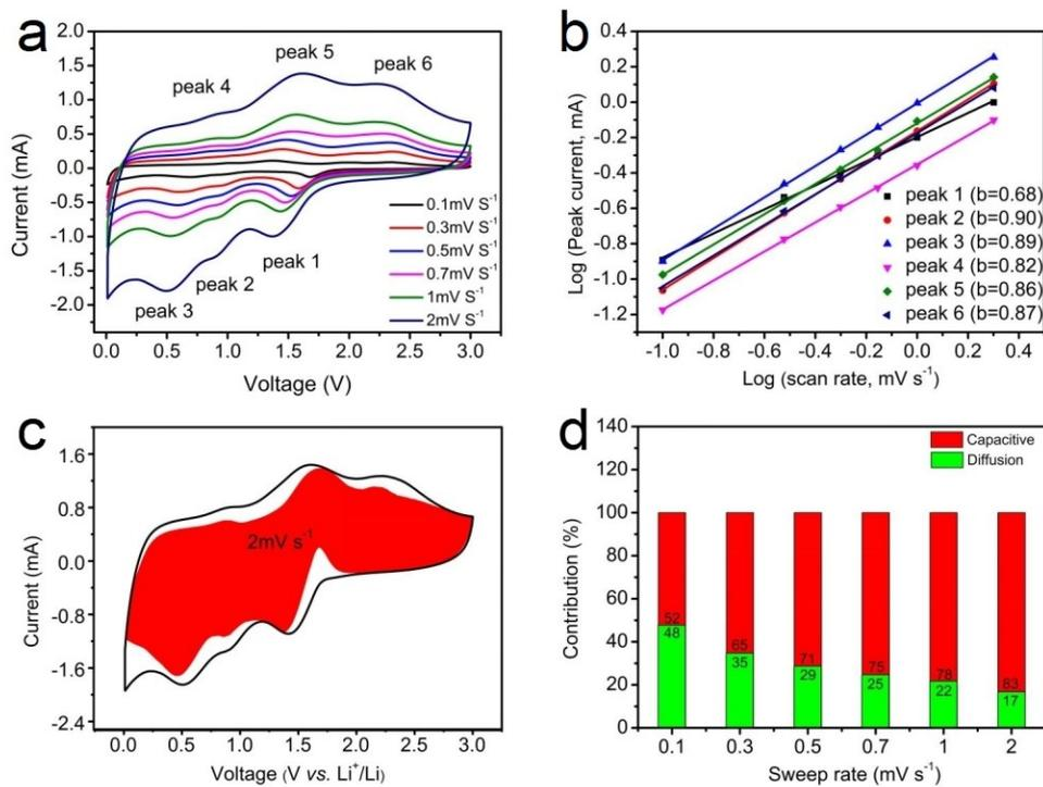
**Figure S7** (a) CV curves of the  $V_2C/NiCo-LDH$  electrode at different scan rates as indicated; (b) Relationship between peak current and scan rate at different scan rates; (c) CV profile at 2  $mV s^{-1}$  with the capacitive contribution (red region); (d) Normalized contribution ratios of the capacitive (red) and diffusion-dominated (green) capacities at various sweep rates based on quantitative analysis.
