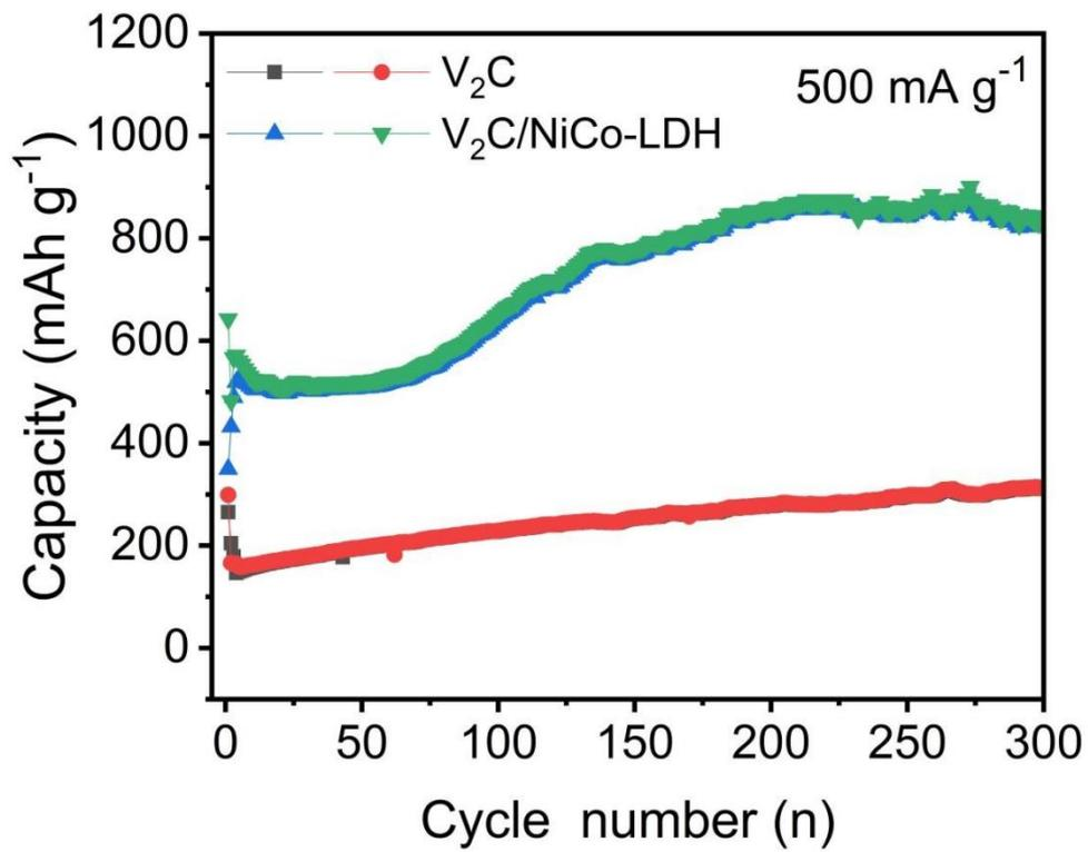
**Figure S6** Cycling behaviors of V<sub>2</sub>C and V<sub>2</sub>C/NiCo-LDH electrodes at 500 mA g<sup>-1</sup>.
