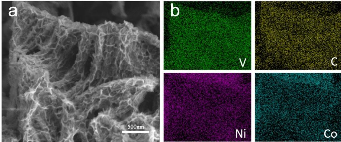
**Figure S3** (a) SEM image of V<sub>2</sub>C/NiCo-LDH hybrids; (b) EDS results of V<sub>2</sub>C/NiCo-LDH hybrids.
