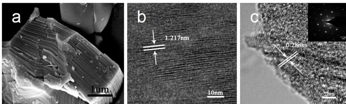
**Figure S2** (a) SEM image of VAl<sub>2</sub>C MAX; (b) TEM and (c) HRTEM images of V<sub>2</sub>C MXene, the inset corresponds to the SAED pattern of V<sub>2</sub>C.
