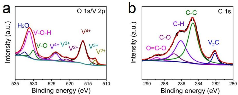
**Figure S1** High-resolution XPS spectra of (a) O 1s/V 2p and (b) C 1s in the V<sub>2</sub>C.
