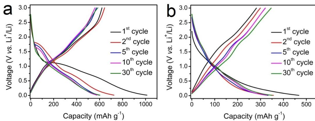
**Figure S4** Selected galvanostatic charge-discharge profiles of the (a)  $V_2C/NiCo-LDH$  and (b)  $V_2C$  electrodes.
