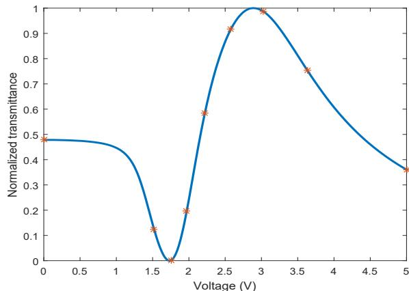
**Fig. S6** Measured voltage-dependent transmittance change curve for **SNUP04** at  $40^\circ\text{C}$ ,  $\lambda = 633\text{ nm}$  and  $1\text{ kHz}$ .
