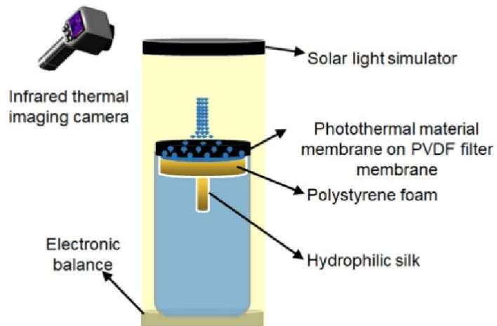
**Figure S6** Schematic illustration of the solar steam generation instrument used in this work.
