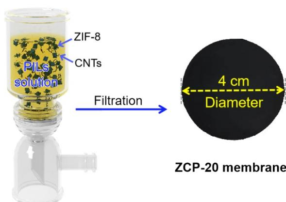
**Figure S3** Picture of ZCP-20 membrane and its dimensions.
