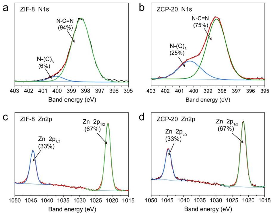
**Figure S5** High-resolution N1s XPS spectra of (a) ZIF-8, (b) ZCP-20, and Zn 2p XPS spectra of (c) ZIF-8 and (d) ZCP-20.
