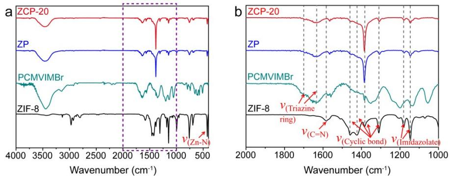
**Figure S4** FT-IR curves of different membranes (a) the complete and (b) enlarged curve.
