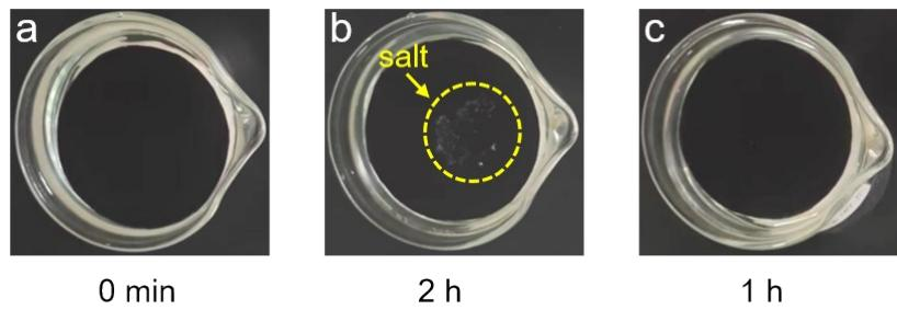
**Figure S7** Water evaporation tests of ZCP-20 membrane for seawater. Please note: there are some crystals on the surface of ZCP-20 membrane after 2 hours under 1 sunlight irradiation (b) and the salt crystals are dissolved within 1 hour in dark (c).
