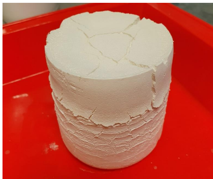
Figure S1. An unmodified MTMS aerogel sample showing cracking
