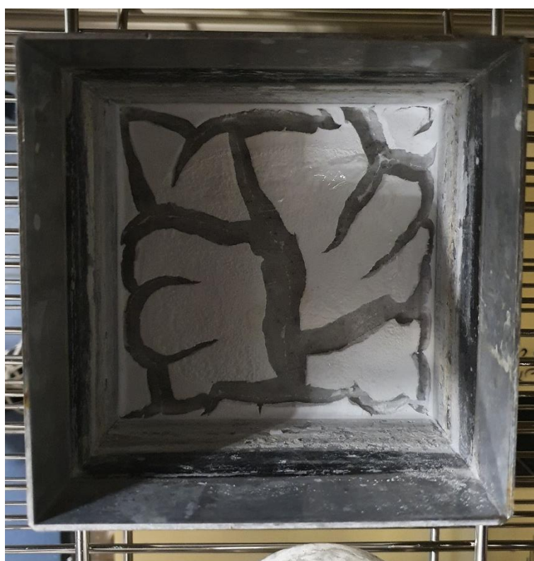
Figure S5. An unmodified MTMS aerogel sample showing cracking
