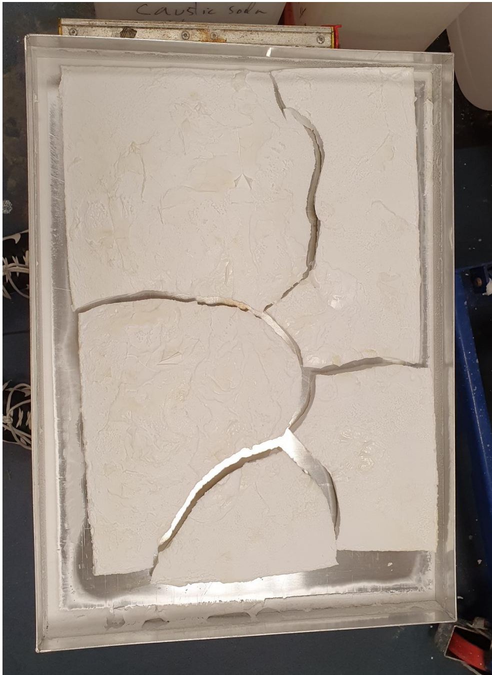
Figure S3. An unmodified MTMS aerogel sample showing cracking
