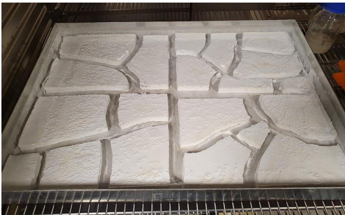
Figure S4. An unmodified MTMS aerogel sample showing cracking
