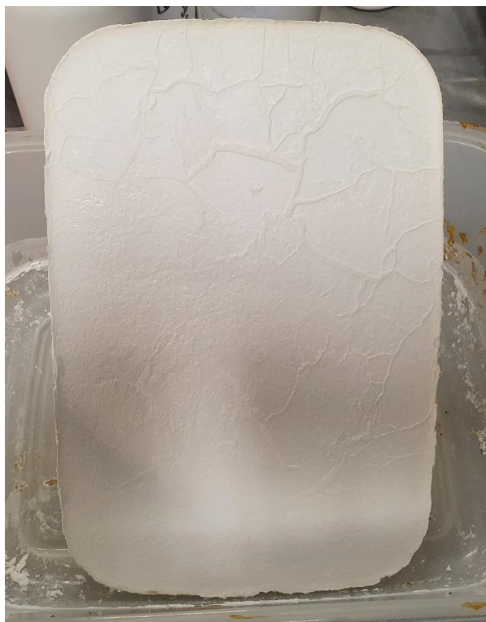
Figure S8. An SRA formed using three repeated recycles of the aerogel material
