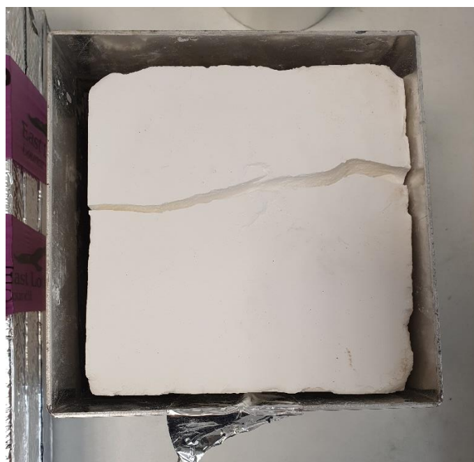
Figure S2. An unmodified MTMS aerogel sample showing cracking
