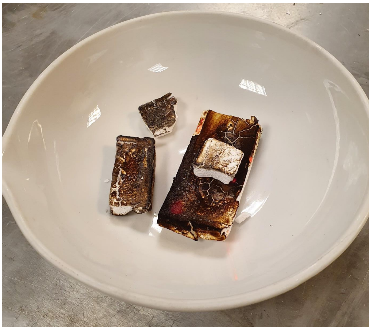
Figure S9. Sample of in tact hydrophilized aerogel sitting on top of a burning hydrophobic aerogel after treatment with a blowtorch
