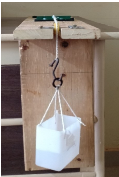
Figure S1: Apparatus for measurement of the spreadability of nanoformulation
