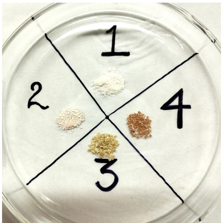
Fig. S1. Moving anti-clockwise, 1,2,3 and 4 depicts synthesized \text{SnO}_2 NPs, 0.1 g \text{SnO}_2 NPs after adsorption of CR dye, completely dried 0.5% \text{SnO}_2@SA beads and completely dried 0.5 % \text{SnO}_2@SA beads after adsorption, respectively.
