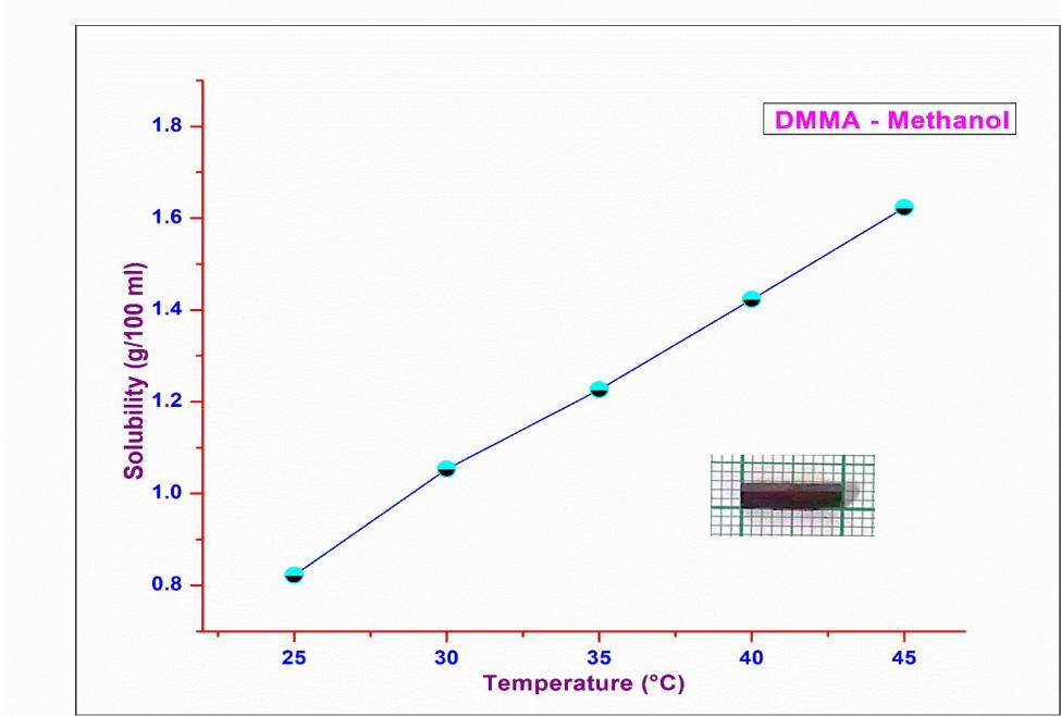
Figure 2: Solubility trace of DMMA and image of the grown crystal
