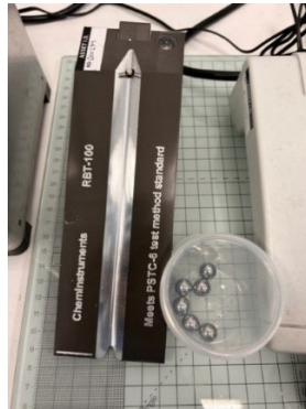
Figure S1. Rolling Ball ramp used to evaluate the tackiness of the cured adhesives.
