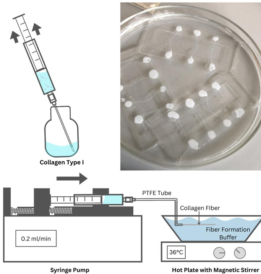
Figure S1: Sample preparation using a syringe pump to extrude collagen type I at a constant rate into a fiber formation buffer placed on a hot plate with magnetic stirrer.
