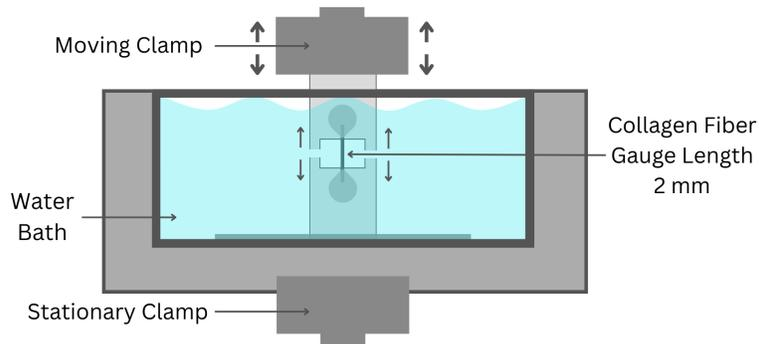
Figure S2: Schematic diagram of a collagen type I fiber glued with cyanoacrylate on test slides with a fixed gauge length of 2 mm and placed in water bath with transparent glass walls made of microscope carrier platelets. The sample holder is clamped inside the tensile testing machine (see ??) and cut to allow the collagen fiber to be stretched vertically.
