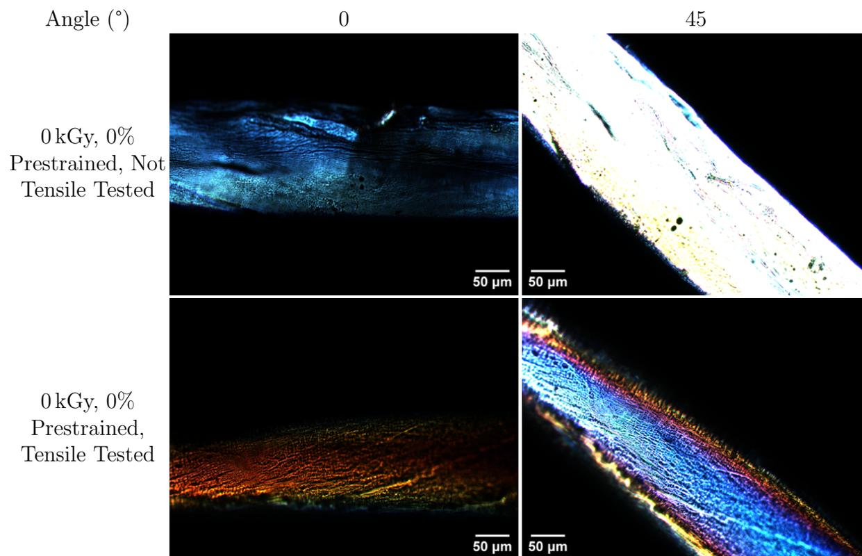
Figure S11: Rotated polarisation microscopy images of non-prestrained and uncrosslinked collagen fibres, before and after the tensile test.
