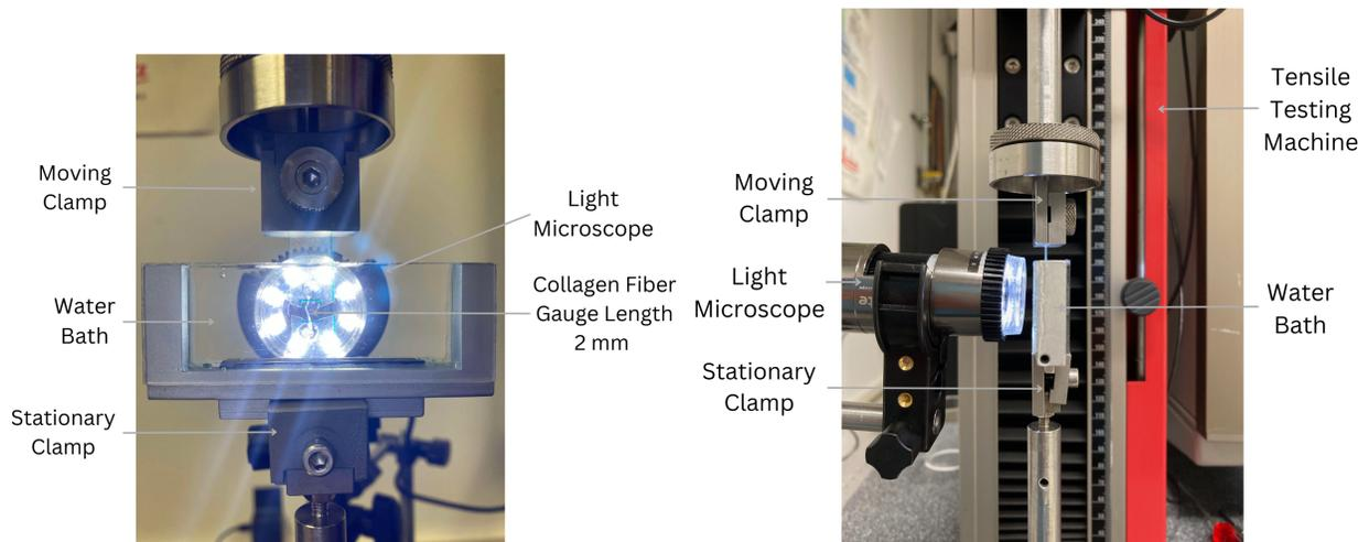
Figure S3: Setup for measuring collagen fibers in a water bath with zwickiLine tensile testing machine (type Z0.5 TS, art. no. 058992, ZwickRoell GmbH & Co. KG, Germany) and DinoLite AM7915MZT microscope (AnMo Electronics Corporation, Taipei, Taiwan) allowing real-time observation and imaging in parallel. The upper clamp moves in y-direction during the measurement (see ??).
