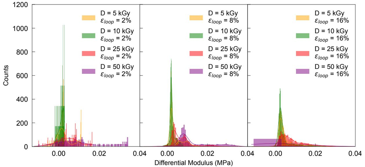
Figure S6: Differential moduli for a prestrain of  $\epsilon_{pre} = 25\%$  for increasing maximal strains in the corresponding loop  $\epsilon_{loop}$  with ten cycles each. The dose  $D$  was achieved in 5 kGy steps.
