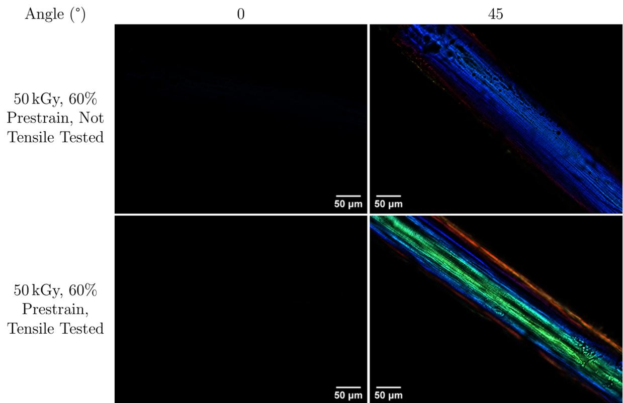
Figure S13: Rotated polarisation microscopy images of prestrained and crosslinked collagen fibres, before and after the tensile test.
