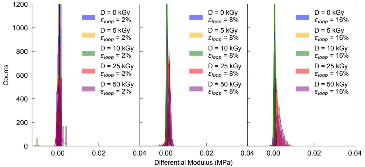
Figure S5: Differential moduli for a prestrain of  $\epsilon_{pre} = 0\%$  for increasing maximal strains in the corresponding loop  $\epsilon_{loop}$  with ten cycles each. The dose D was achieved in 5 kGy steps.
