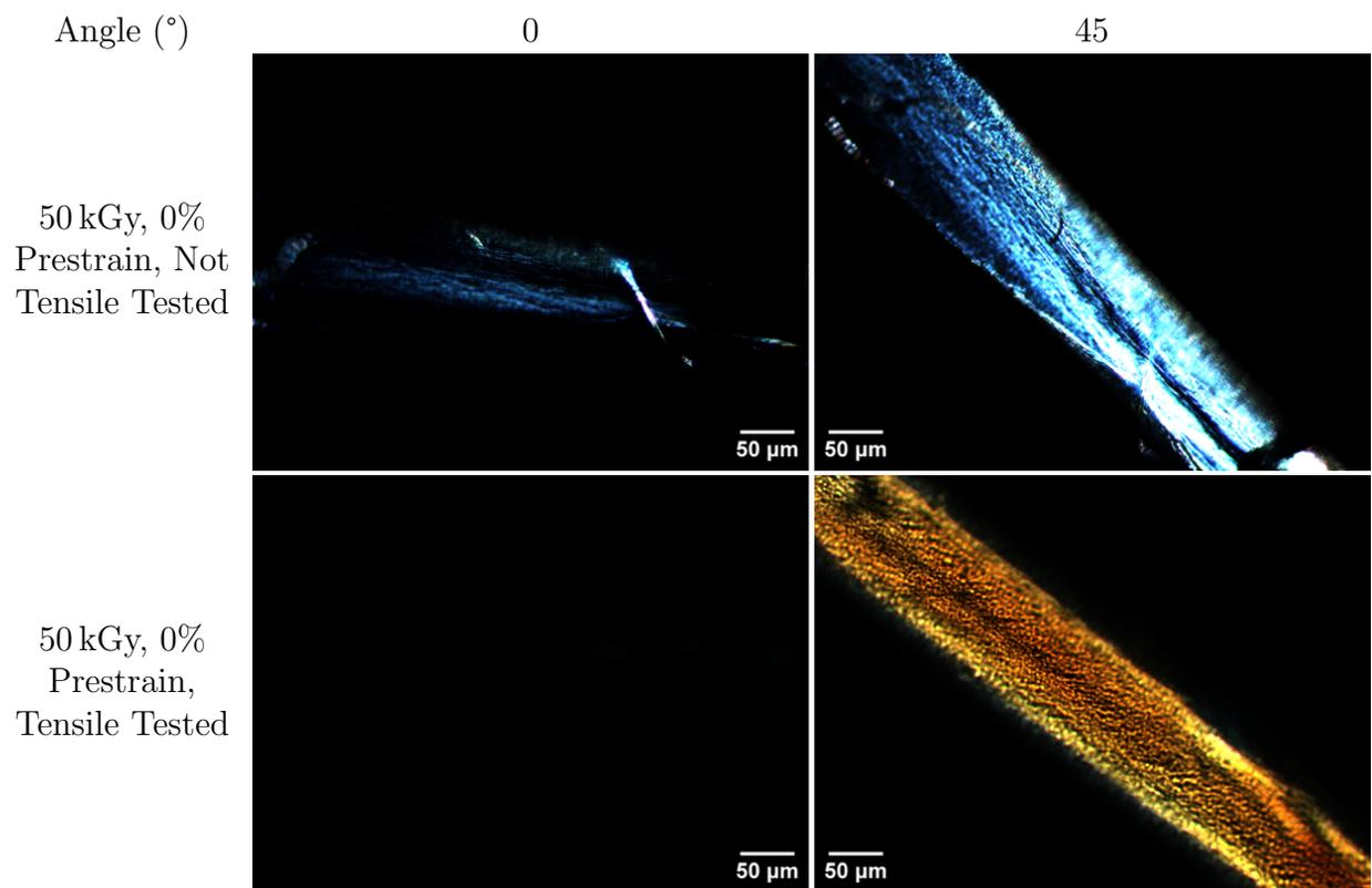
Figure S12: Rotated polarisation microscopy images of non-prestrained collagen fibers crosslinked with 50 kGy, before and after the tensile test.
