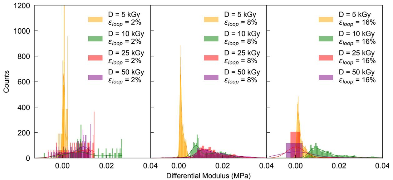
Figure S7: Differential moduli for a prestrain of  $\epsilon_{pre} = 60\%$  for increasing maximal strains in the corresponding loop  $\epsilon_{loop}$  with ten cycles each. The dose  $D$  was achieved in 5 kGy steps.
