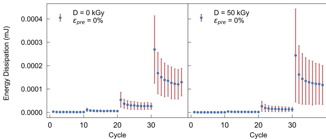
Figure S8: Energy dissipation  $\Delta E \approx W$  within a single measurement cycle, i.e. stretching and retracting the fiber sample once within a defined strain range. Shown are the mean values for unirradiated and irradiated collagen fibers without prestraining  $\epsilon_{pre}$ . A higher irradiation dose  $D$  does not initially appear to have a particularly large effect on energy dissipation.
