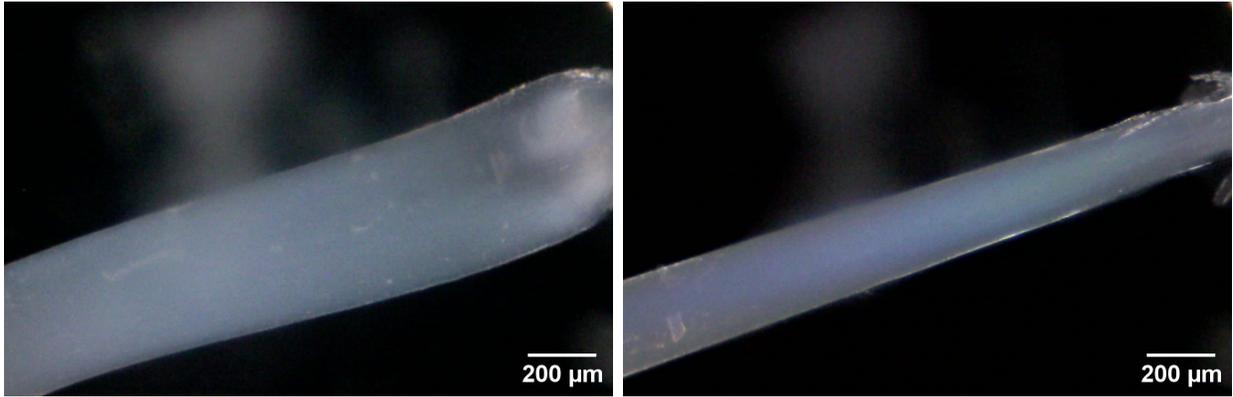
Figure S4: A fully hydrated collagen fiber exemplary imaged with DinoLite light microscope before tensile test (left) and after tensile test (right).
