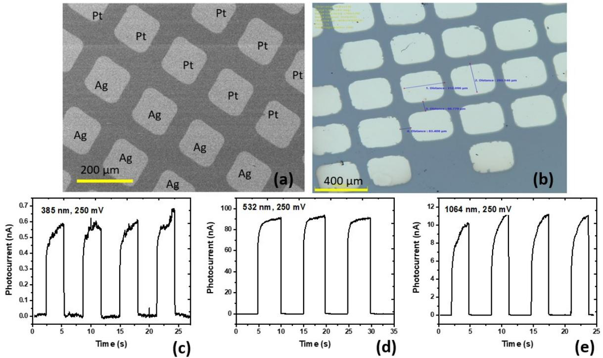
**Figure S1.** (a) Optical image of the device Si/SnSe, (b) Si, (c) photodetection of the bare n-Si device under 385, (d) 532, and (e) 1064 nm at 250 mV bias.
