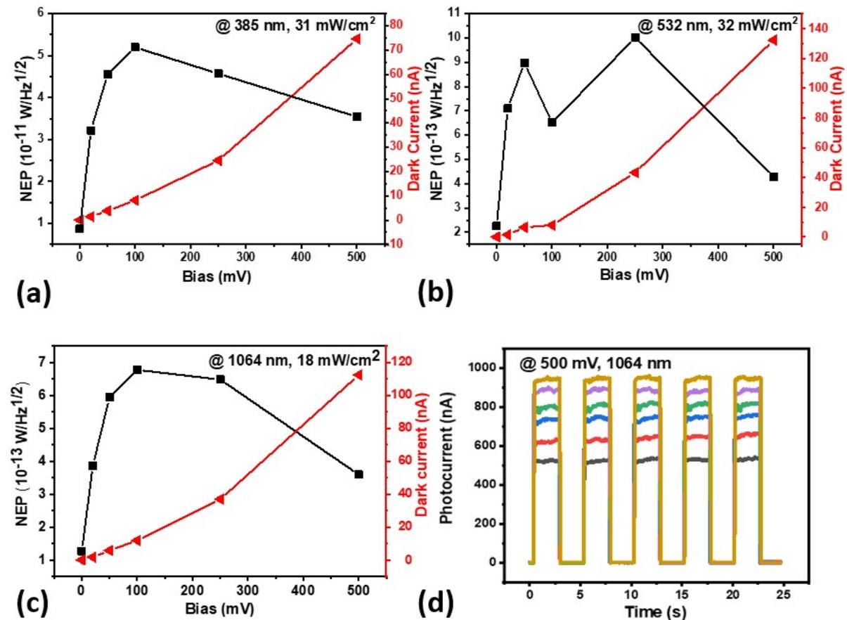
**Figure S2.** NEP and dark current at (a) 385 nm, (b) 532 nm, (c) 1064 nm, and (d) photocurrent at different power densities at 1064 nm laser at 500 mV bias.
