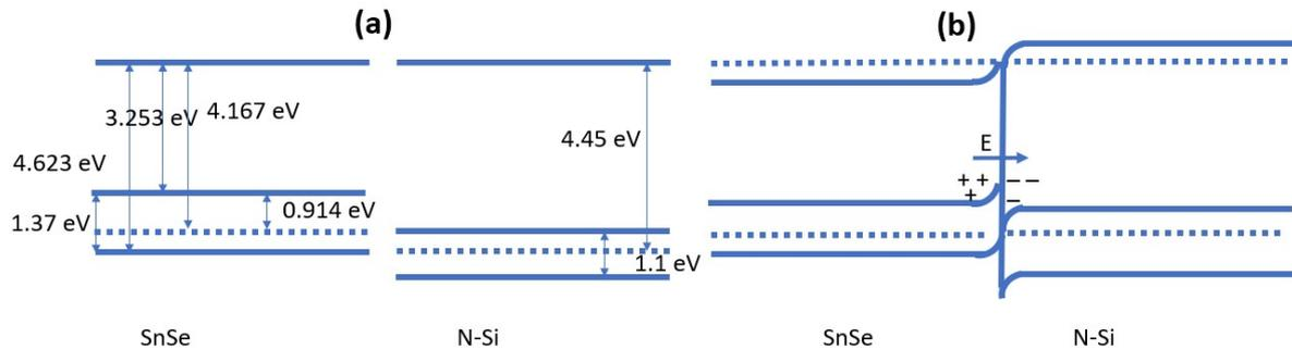
**Figure S6.** Energy band alignment of the n-Si and SnSe (a) before and (b) after deposition.
