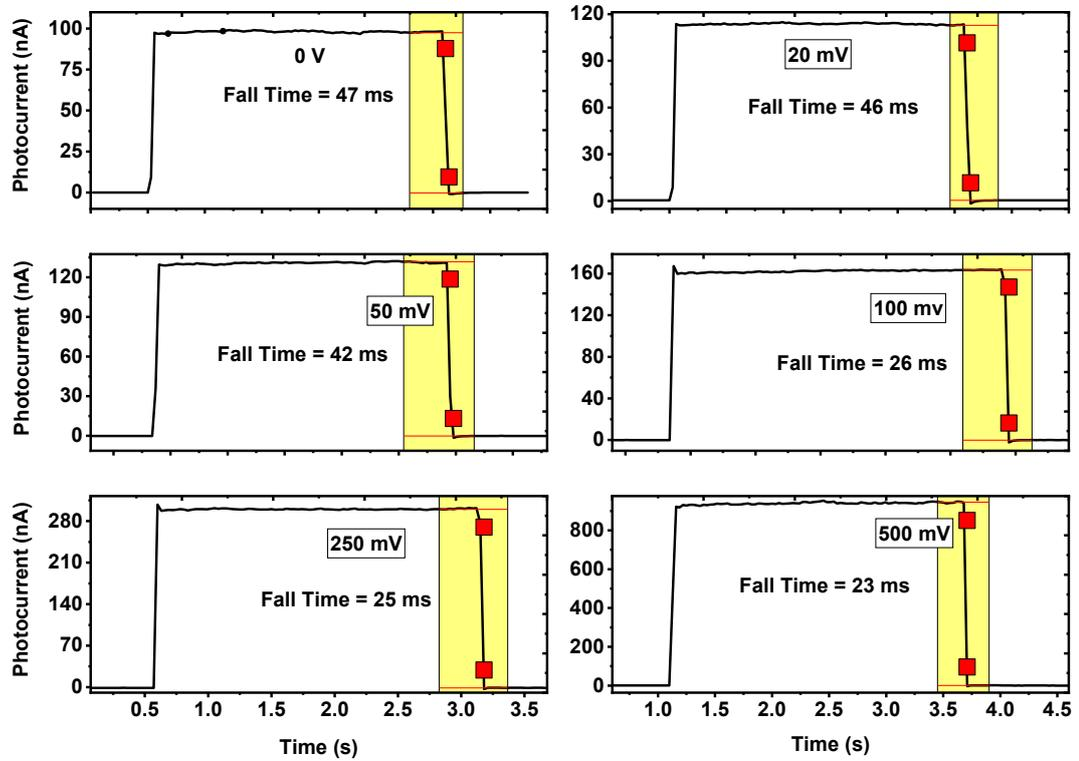
**Figure S5.** Recovery time of the device under different voltages at 18 mW/cm<sup>2</sup> power density.
