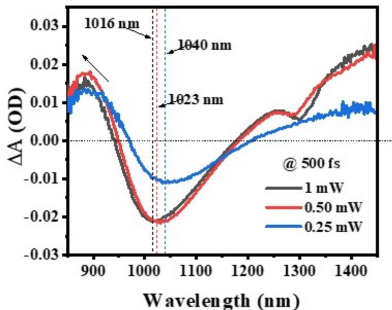
**Figure S4.** Comparative transient spectra at different fluences.
