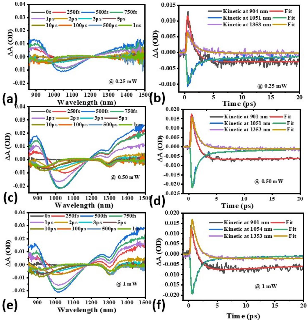
**Figure S3.** Transient spectra (differential absorption) and their kinetics at different fluences (a), (b) for 0.25 mW, (b), (c) 0.50 mW, and (d) and (e) 1 mW.
