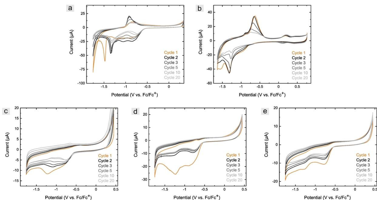
Fig. S16 Cyclic voltammetric investigation of a,b,c) PS-ox@Fc-2 and d) PSOH@Fc-2 and e) PSDVB@PFMMA-1 based ceramics synthesized in a,b) synthetic air or c-e) nitrogen atmosphere. The measurements in c-e) were carried out in alkaline solution (1 M NaOH) and a,b) were measured in 0.1 M NaClO<sub>4</sub> with a scan rate of 20 mV s<sup>-1</sup>. The 1, 2, 3, 5, 10, and 20 cycles were shown, respectively.
