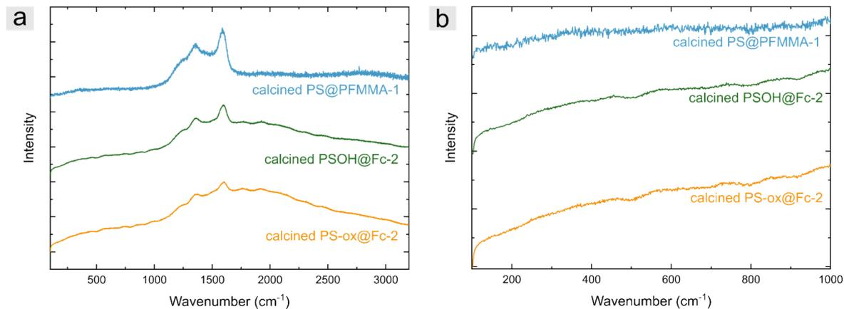
Fig. S13 Raman spectroscopy data of calcined particles in nitrogen atmosphere until 580 °C. a) Overview between 100 and 3200  $\text{cm}^{-1}$ , b) partial spectrum between 100 and 1000  $\text{cm}^{-1}$ , where the iron oxide signals could be expected.
