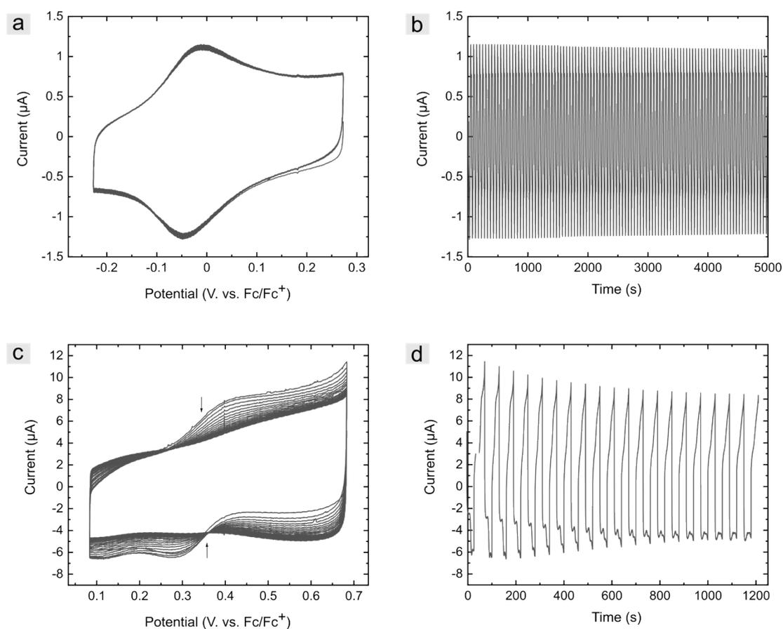
**Fig. S7** Cyclic voltammetric investigations of a,b) PS-ox@Fc-2 (50 cycles) and c,d) PSOH@Fc-2 (20 cycles) in aqueous NaClO<sub>4</sub> (0.1 M) with a scan rate of 20 mV s<sup>-1</sup>.
