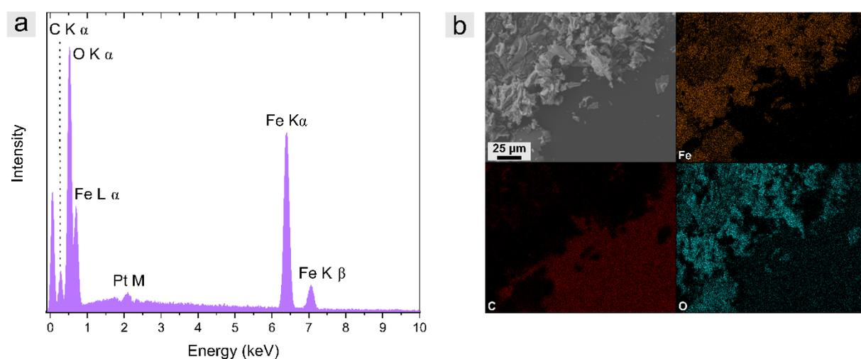
Fig. S10 Energy dispersive X-ray spectra of PFMA-based ceramics (mean values (wt-%) of 3 measurement results: C:  $12 \pm 4$ , O:  $29 \pm 4$ , Fe:  $57 \pm 1$ , Pt:  $1 \pm 1$ ) and corresponding mapping images of the ceramic synthesized in synthetic air up to 580 °C.
