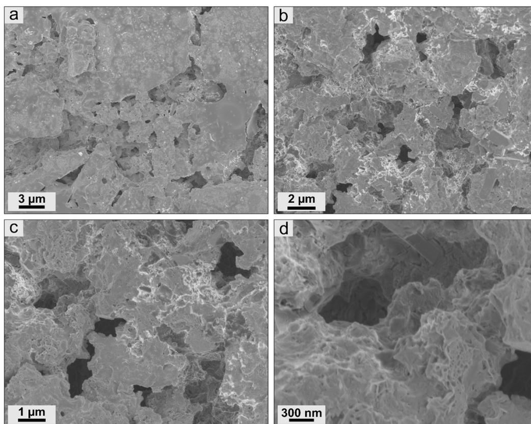
Fig. S11 Scanning electron micrographs of calcined PFMMA in nitrogen atmosphere up to 580 °C.
