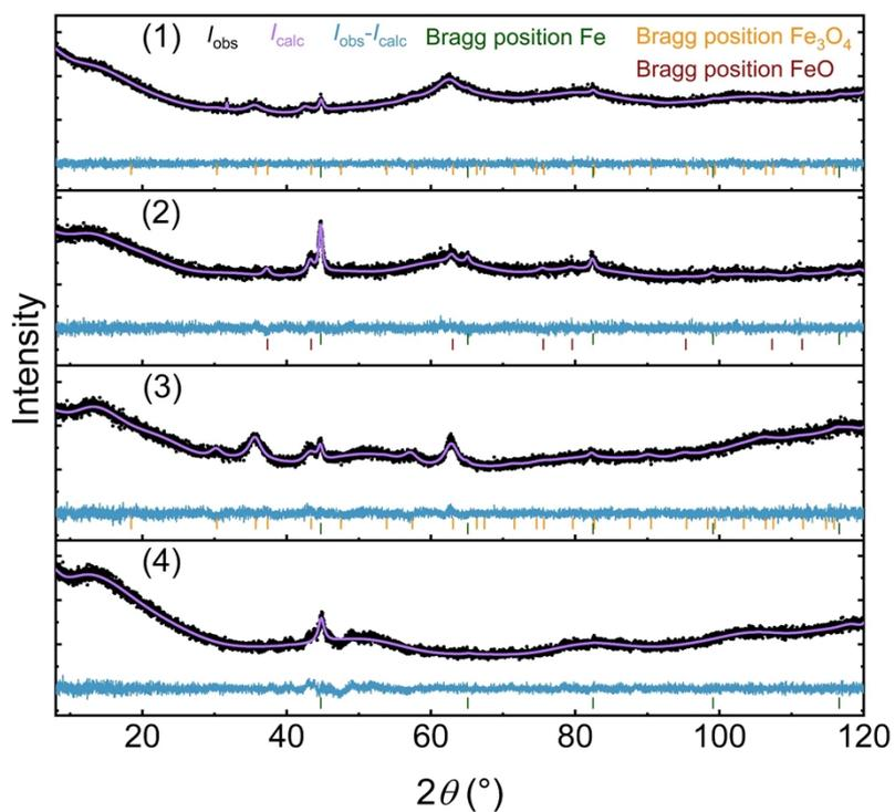
Fig. S12 X-ray diffractogram of calcined (1) PFMMA, (2) PSDVB@PFMMA-1, (3) PSOH@Fc-2, and (4) PS-ox@Fc-2 particles synthesized under nitrogen atmosphere.
