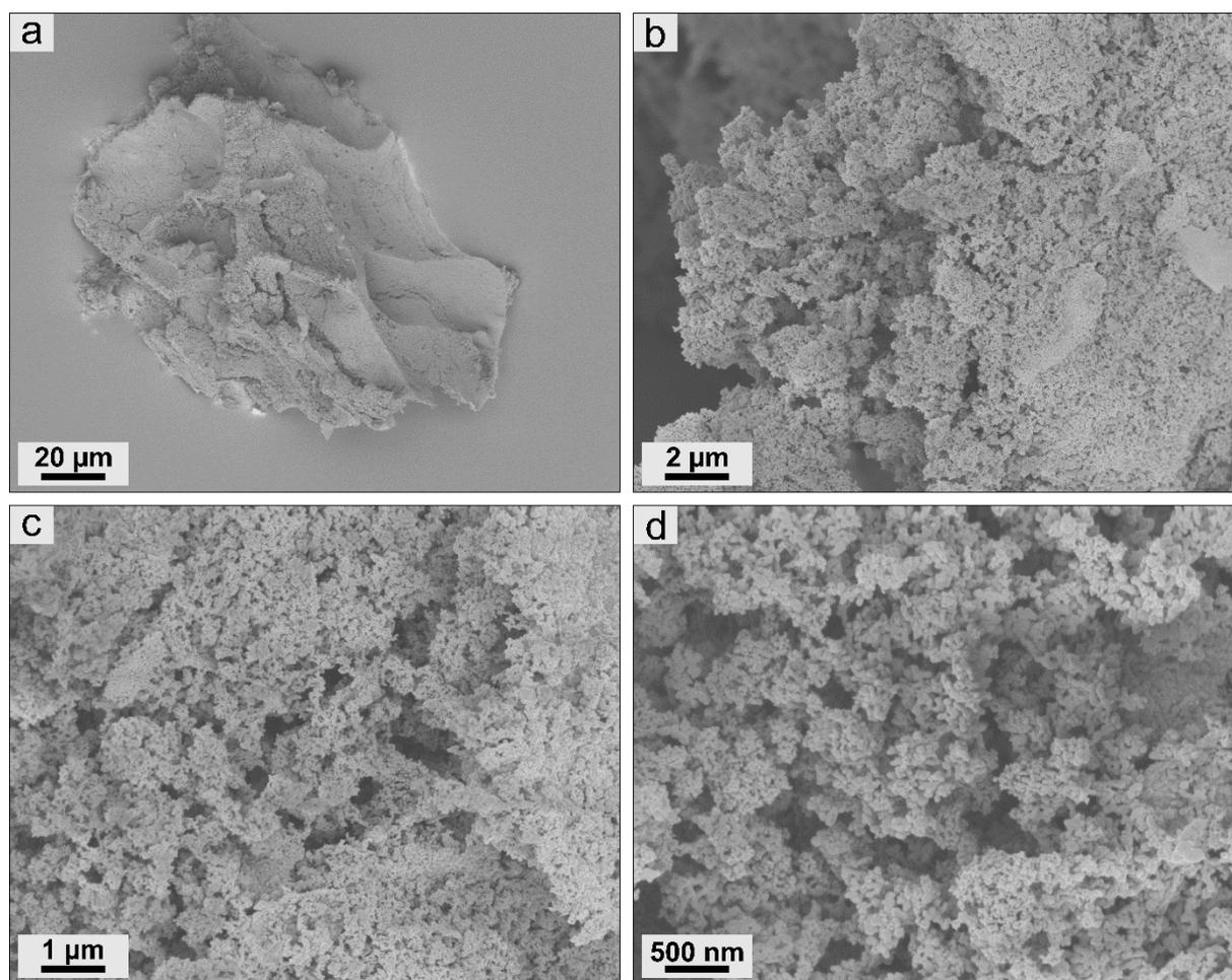
Fig. S9 Scanning electron micrographs of calcined PFMA in synthetic air up to 580 °C.
