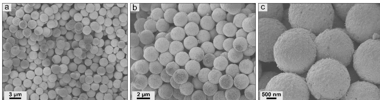
**Fig. S8** Additional scanning electron micrographs of PSDVB@PFMMA-1 based ceramics synthesized under nitrogen atmosphere.
