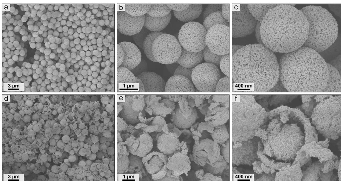
Fig. S15 Scanning electron micrographs of calcined a-c) PSDVB@PFMMA-5 and d-f) PSDVB@PFMMA-6 prepared in synthetic air up to 580 °C.
