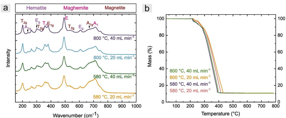
**Fig. S14** a) Raman and b) thermogravimetric analyses of PSDVB@PFMMA-2 based ceramics synthesized under synthetic air in different gas flows and until different maxima temperatures.
