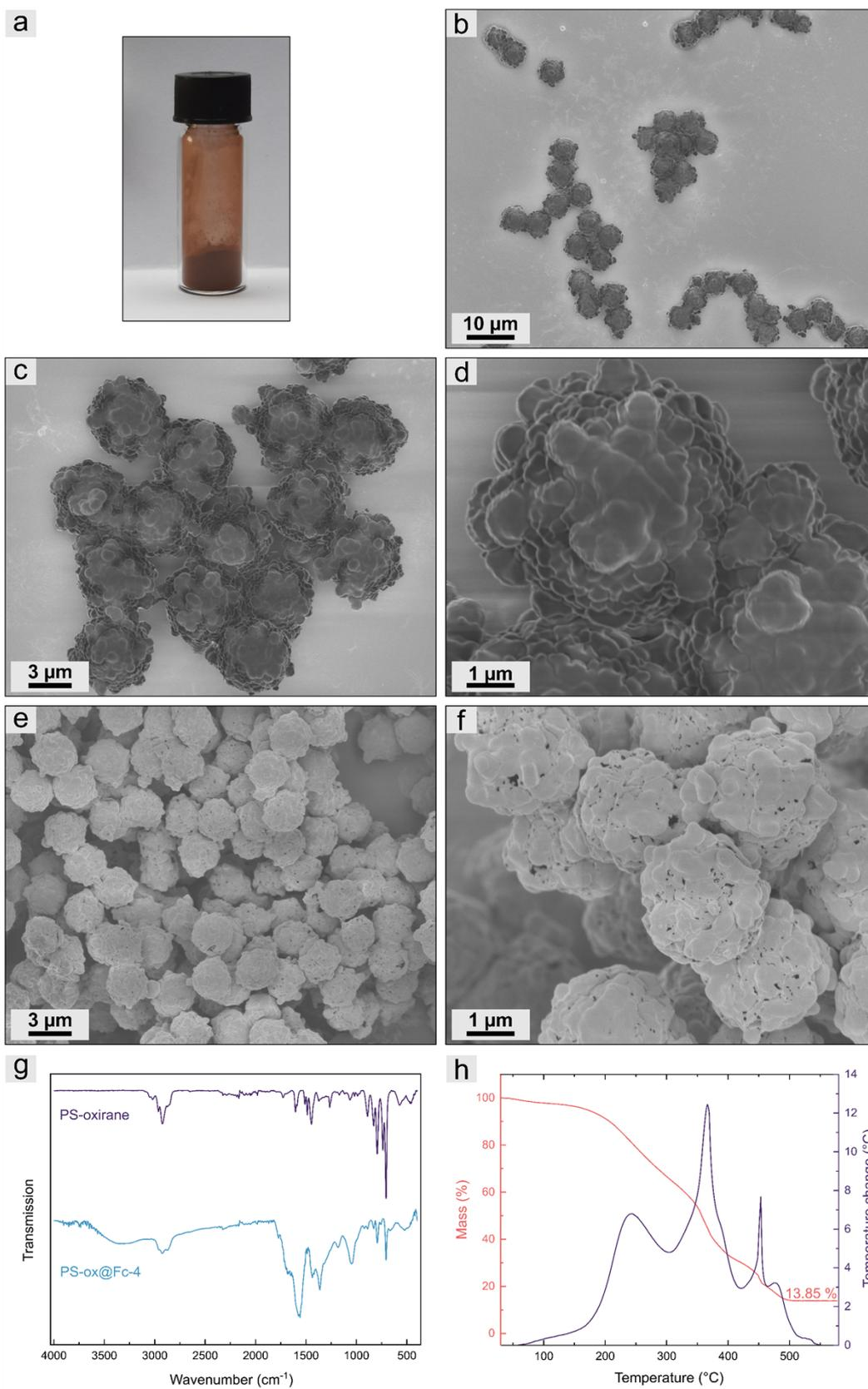
**Fig. S2** a) Image of PS-ox@Fc-4 synthesized in THF, corresponding scanning electron micrographs b-d) of the precursors and e,f) the ceramics prepared in synthetic air up to 580 °C. g) Infrared spectroscopic data of PS-ox@Fc-4 and PS-oxirane and h) thermogravimetric analysis of PS-ox@Fc-4.
