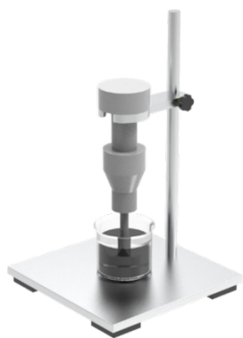
Dispersion of MWCNT/THF(BHT 750 ppm)
