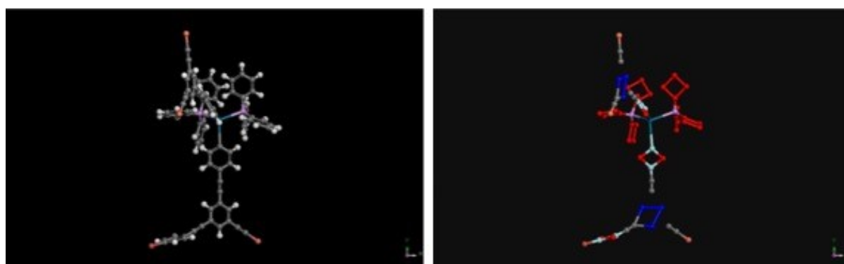
Figure S36. Structure of the all-atom (left) and mapped coarse-grain (right) polymer fragment 15. Key: C – grey, H – white, Cu – orange, tBER grain – bright blue, Pd – dim blue, P – purple, BER grain – red, Br – burgundy, dBER grain – pale blue.
