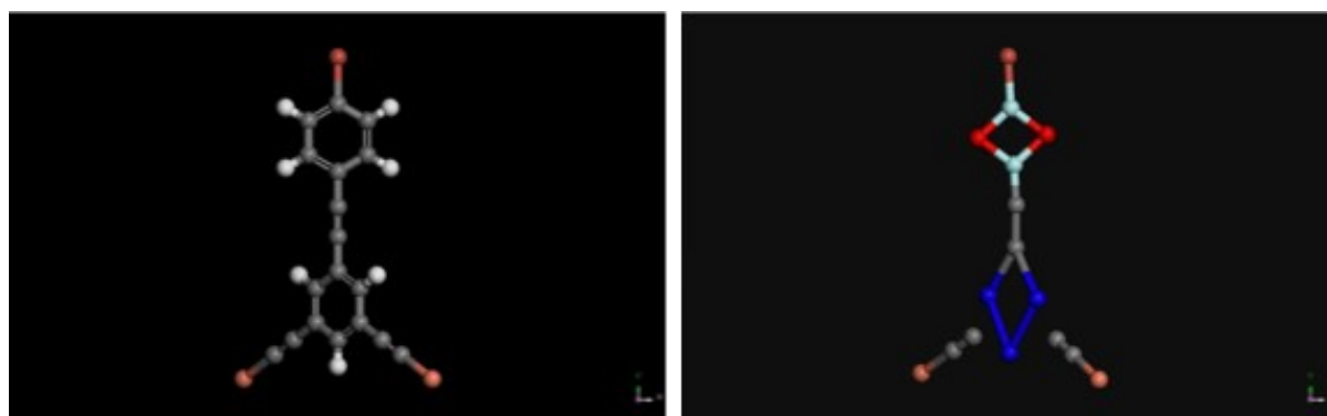
Figure S24. Structure of the all-atom (left) and mapped coarse-grain (right) polymer fragment 3. Key: C – grey, H – white, Cu – orange, tBER grain – bright blue, BER grain – red, Br – burgundy, dBER grain – pale blue.
