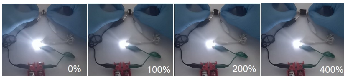
Fig. S10. The brightness variation of a LED lamp when the CAGA acting as an electrical conductor in closed circuit during stretching process, showing unchanged brightness from 100% to 400% tensile strain.
