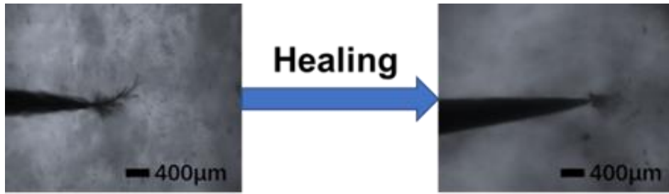
Fig. S18. The optical images of EP-CB before and after healing for electrical trees. After healing at 180 °C/15 MPa for 30 min, the electrical channels in EP-CB were partially healed as damage can be still observed.
