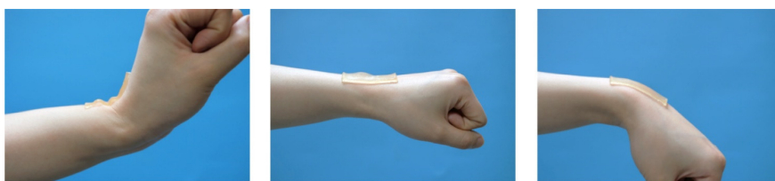
Fig. S39. A piece of stretchable pAd-TENG-based e-skin can attach and conform to a human external wrist even under a large tilting action.
