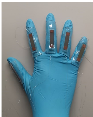
Fig. S12. Photograph of wide-range metal film-based strain sensors attached to five fingers.
