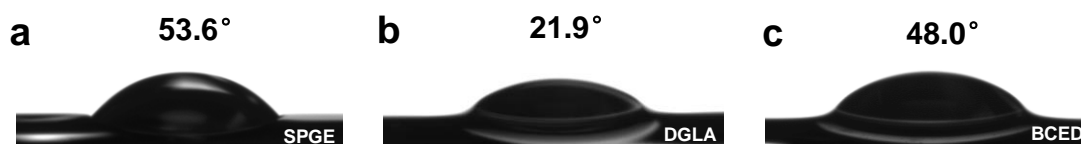
Fig. S19. Surface contact angle images of the water droplet to (a) SPGE, (b) DGLA, and (c) BCED layers in air.
