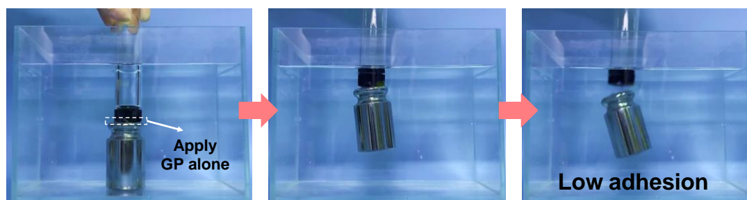
Fig. S3. Digital images showing the poor underwater adhesion capability of GP liquid.
