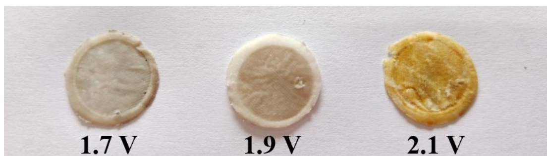
Fig. S4. Optical photos of the fiberglass separators at different charge cut-off voltages.
