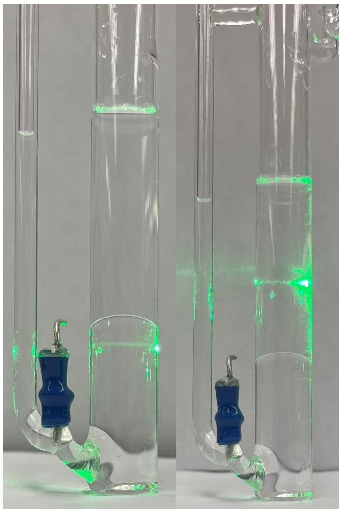
Figure S1: Glass cell Images of a two-phase system over the course of 5 min. A 3 mL aqueous top layer containing 0.1 M [\text{NBu}_4][\text{Cl}] was pipetted over 3 mL of DCE containing 0.1 M [\text{NBu}_4][\text{PF}_6] . No emulsification was observed after 5 minutes of the two phases being in the presence of one another.
